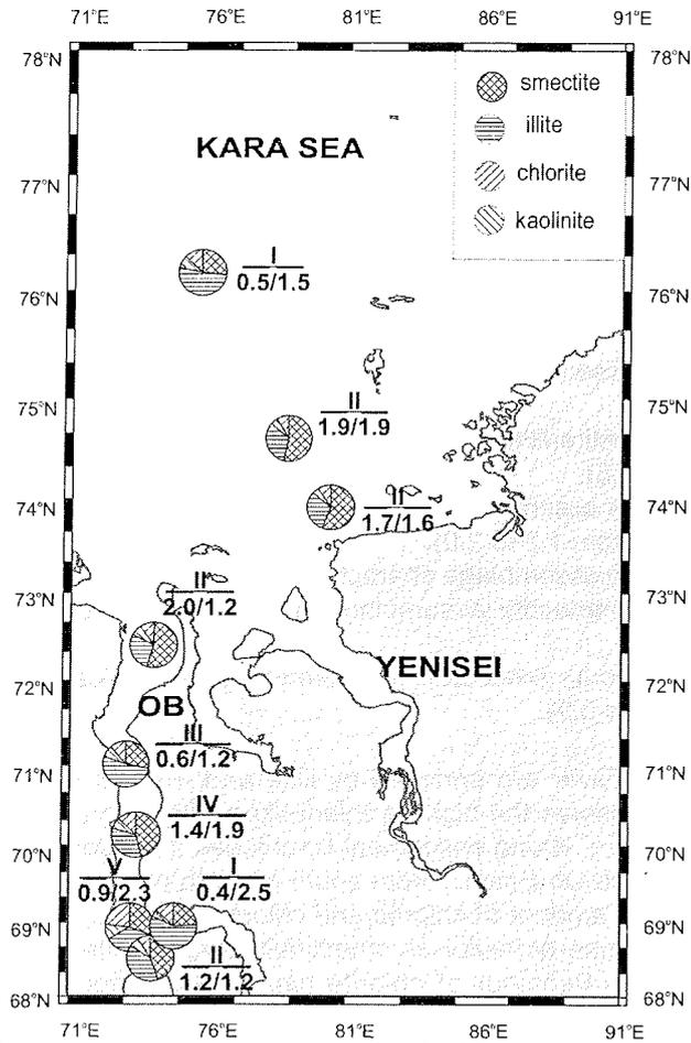
Figure 7-4: Clay-mineral assemblages (rel. %) of BP02 surface sediments. Roman numerals – assemblage types. In denominator: left fraction – Sm/III ratio, right fraction – Chl/Kaol ratio.
