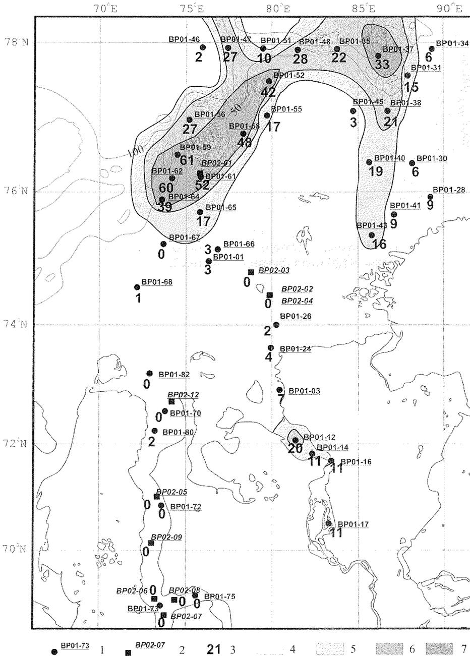
Figure 7-3: Distribution of black ore minerals in fraction >125 μm. 1 – BP01 stations; 2 – BP02 stations; 3 – amount of black ore minerals (biogenic-free, rel. %); 4 - <10 rel. %; 5 – 10-20 rel. %; 6 – 20-30 rel. %; 7 - >30 rel. %.
