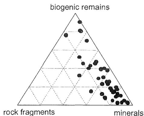
Figure 7-1: Composition of fraction  $>125 \mu\text{m}$  from the eastern Kara Sea surface sediments (BP01 data, rel. %).
