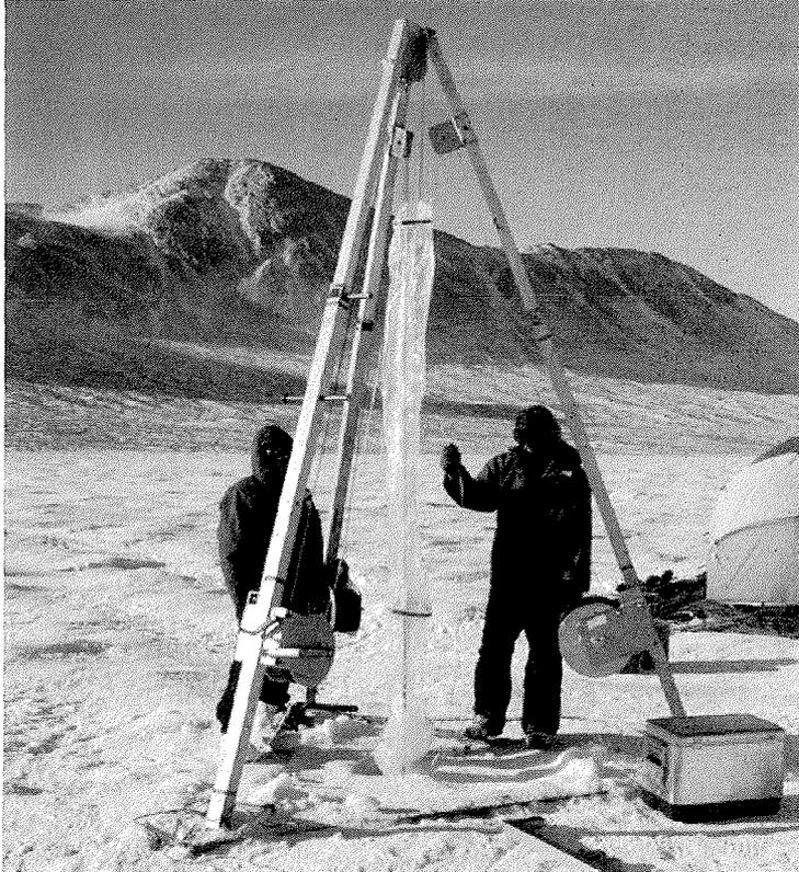
**Fig. 2.8:** Coring tripod on Lake Fryxell. In the center is the tubular film visible, which coats the subaquatic coring equipment to the lake bottom.
