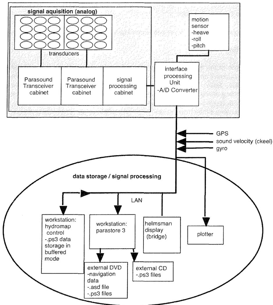
**Figure 7.2:** Software and hardware configuration of the PARASOUND system on RV "Akademik Boris Petrov": Connection diagram of different system components.
