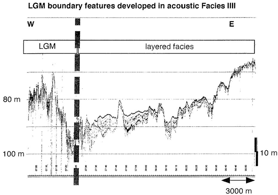
**Figure 7.14:** Glacial facies neighbouring thick sediment sequences of probably fluvial originated sediments. The layered sediments seem to border to the glacial influenced facies. There is a distinct change in the relief energy, the glaciated terrain being more hummocky. The acoustic layered facies seems to accumulate in depressions.
