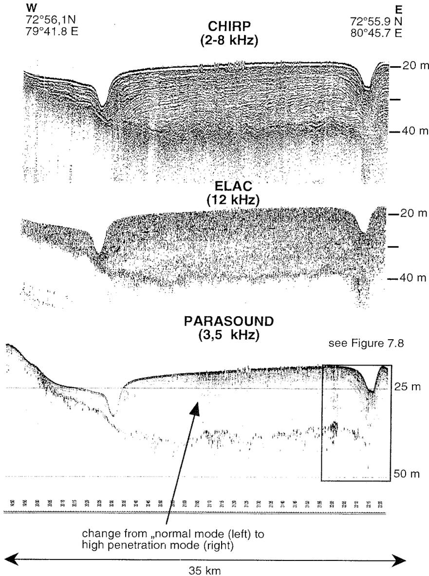
**Figure 7.4:** Comparison of different Echosounding systems used during several expeditions of the SIRRO project (CHIRP (Niessen and Dittmers 2001) and ELAC system (Weiel & Stein 1999, Dittmers & Stein 2000, Niessen & Dittmers 2001)).
