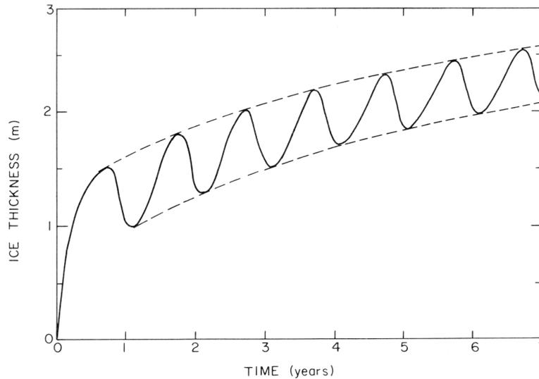
**Figure 1.5:** The thermodynamic growth of sea ice thickness is limited by the oceanic heat flux and the thermal conductivity of the ice. [from *Maykut*, 1986, Fig. 11]
