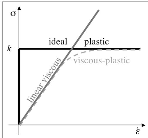
**Figure 2.1:** Schematic of different mechanical behaviour approximations for sea ice [after *Hibler*, 1979; *Mellor*, 1986].
