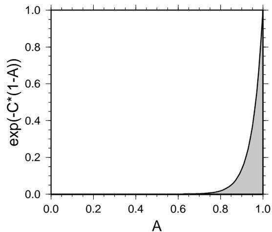
**Figure 2.2:** Exponential relationship of ice strength  $P$  and ice concentration  $A$  (see Equation (2.22));  $C^* = 20$ .
