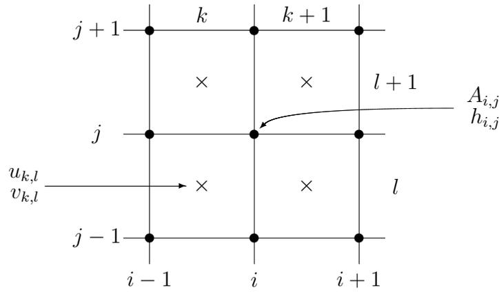
**Figure 2.4:** The Arakawa B arrangement of variables on a regular grid. The positions for scalar variables are labelled with indices  $i$  and  $j$  and marked with a '•', and those of both vector components bear labels  $k$  and  $l$  as well as the mark '×'. For the consecutive numbering of the indices  $i = k$  and  $j = l$  holds true.
