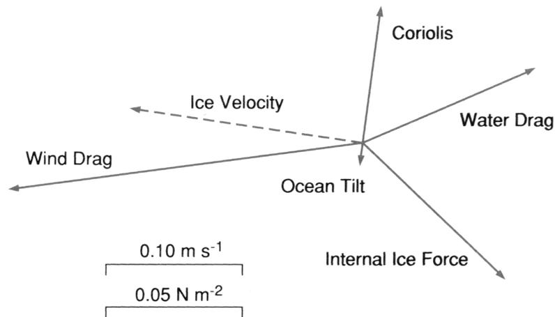
**Figure 1.7:** Schematic diagram of the momentum balance of sea ice for winter conditions based on wind and water stress measurements. The internal force is derived as a residual and the resulting ice velocity is shown as a dashed line. [from *Hibler and Flato*, 1992, Fig. 12.1]
