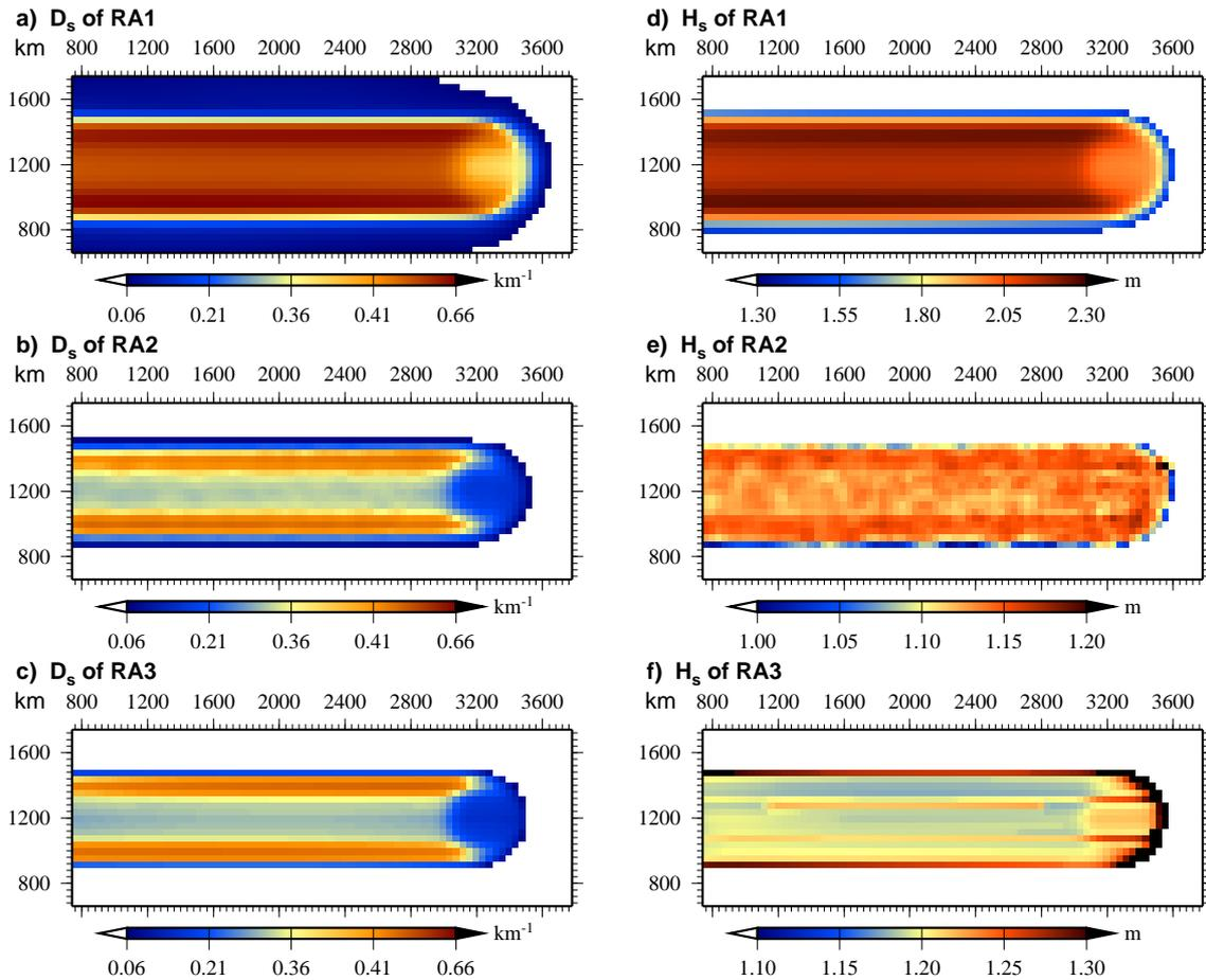
**Figure 7.3:** (a–c) Sail density  $D_s$  and (d–f) sail height  $H_s$  of all three ridge algorithms as caused by the moving cyclone on a grid with no topography. The initial ice concentration was 0.95 and the initial ice thickness 0.5 m.
