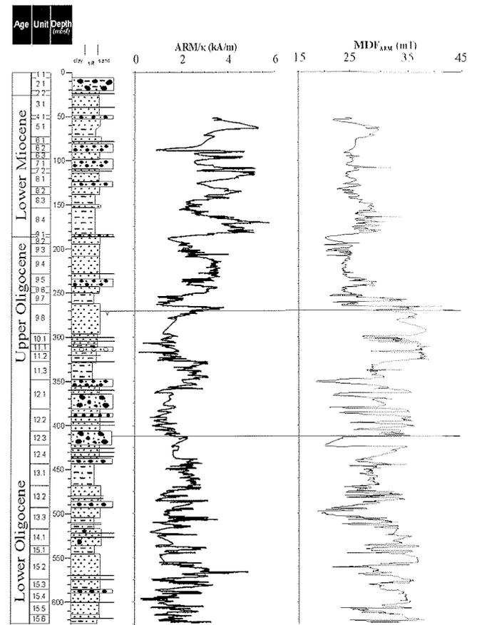
Fig. 5 – Down-core variations of ARM/ $k$  and  $MDF_{ARM}$  for CRP-2/2A. The lines at 270 and 413 mbsf indicate the boundaries between intervals with different magnetic properties.
