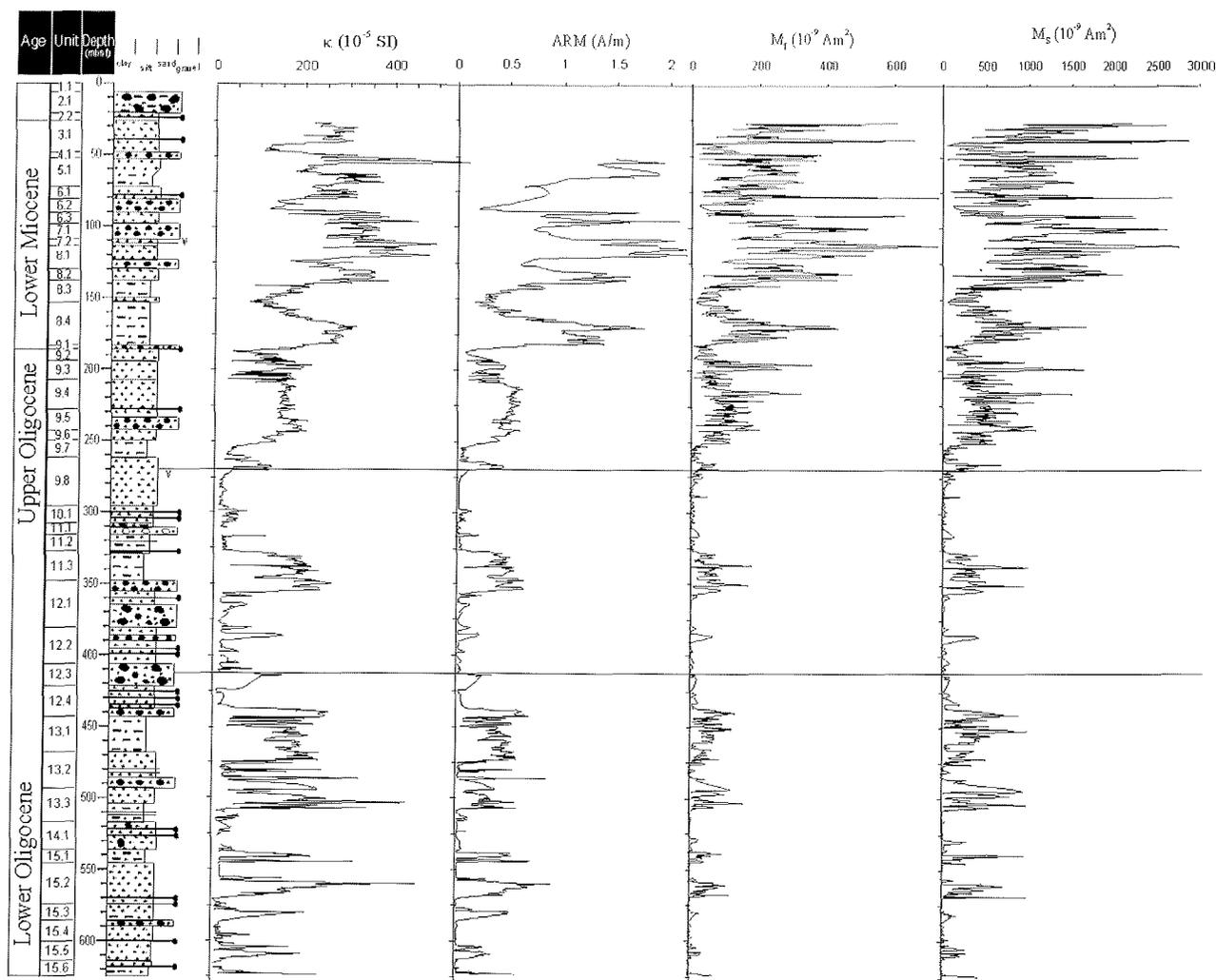
Fig. 1 – Down-core variation of ferrimagnetic concentration-dependent parameters ( $\kappa$ , ARM,  $M_1$  and  $M_2$ ) in CRP-2/2A. The lines at 270 and 413 mbsf indicate the boundaries between intervals with different magnetic properties (see discussion in text, Fig. 2 & Tab. 1).
