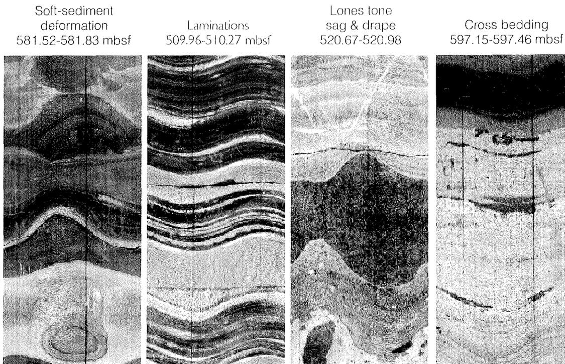
Fig. 1 - Processes affecting CRP-2 bedding dips are illustrated in these four core images. Each image is an unwrapped 360° scan of the outer core surface, so planar features are evident as sinusoids. Soft-sediment deformation (left image) and lonestones (dark patches at the center and bottom of the third image) are generally non-planar and therefore non-sinusoidal in these scans. The two vertical lines in each image are reference lines drawn on the core.
