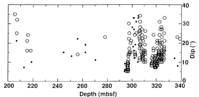
Fig. 7 - A portion of the whole-core bedding dip dataset of figure 3, displaying the interval 200-340 mbsf. These data are compatible with the hypothesis of an angular unconformity at about 300 mbsf, but they are inconclusive.
