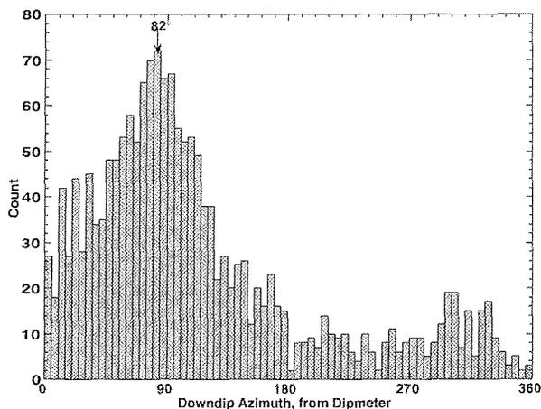
Fig. 4 - Histogram of all downdip azimuths determined by dipmeter. The strong peaking at  $82^\circ$  is attributable mainly to structural dip.
