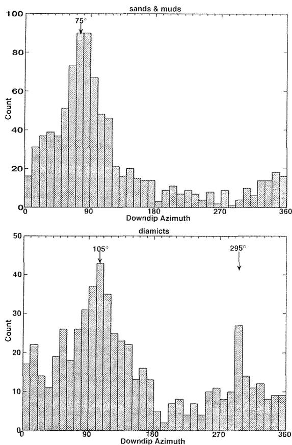
Fig. 10 - Histograms of downdip azimuths determined by dipmeter. Data for sands and muds (top) are plotted separately from those for diamict-dominated lithologies (bottom).
