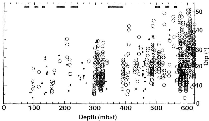
Fig. 3 - Identifications of bedding dip on whole-core scan images. Open circles are picks classified as fair/good; solid dots are dubious picks. Solid vertical bars indicate intervals that were not analyzed. Note the high dip dispersion and the gradual increase in dips downhole.
