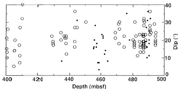
Fig. 8 - A portion of the whole-core bedding dip dataset of figure 3, displaying the interval 400-500 mbsf. These data do not confirm dipmeter-based evidence of an angular unconformity within the interval 440-479 mbsf.
