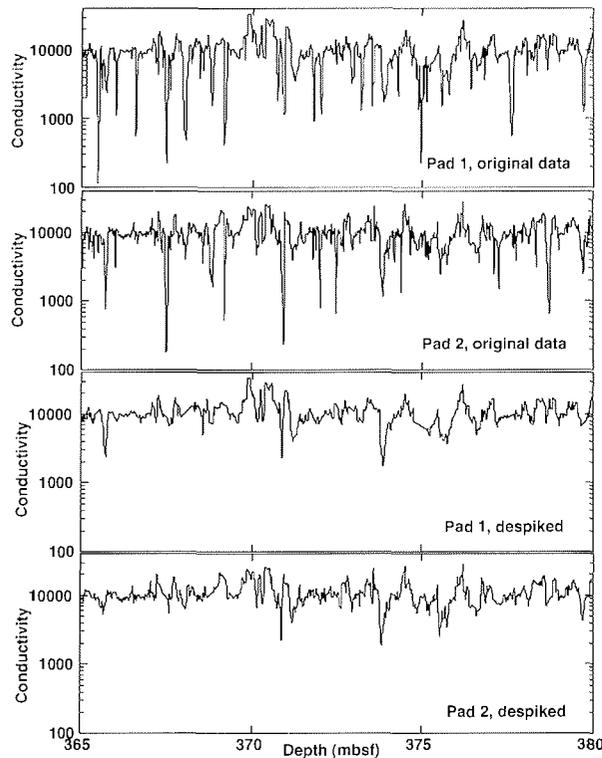
Fig. 2 - Short intervals from two of the four microconductivity traces recorded by the dipmeter. Lonestones cause frequent spikes to low conductivity. Because most lonestones are too small to be detected on more than one pad, they degrade trace coherence among pads. Application of a despiking algorithm (bottom two traces) minimizes this problem and improves reliability of correlations.
