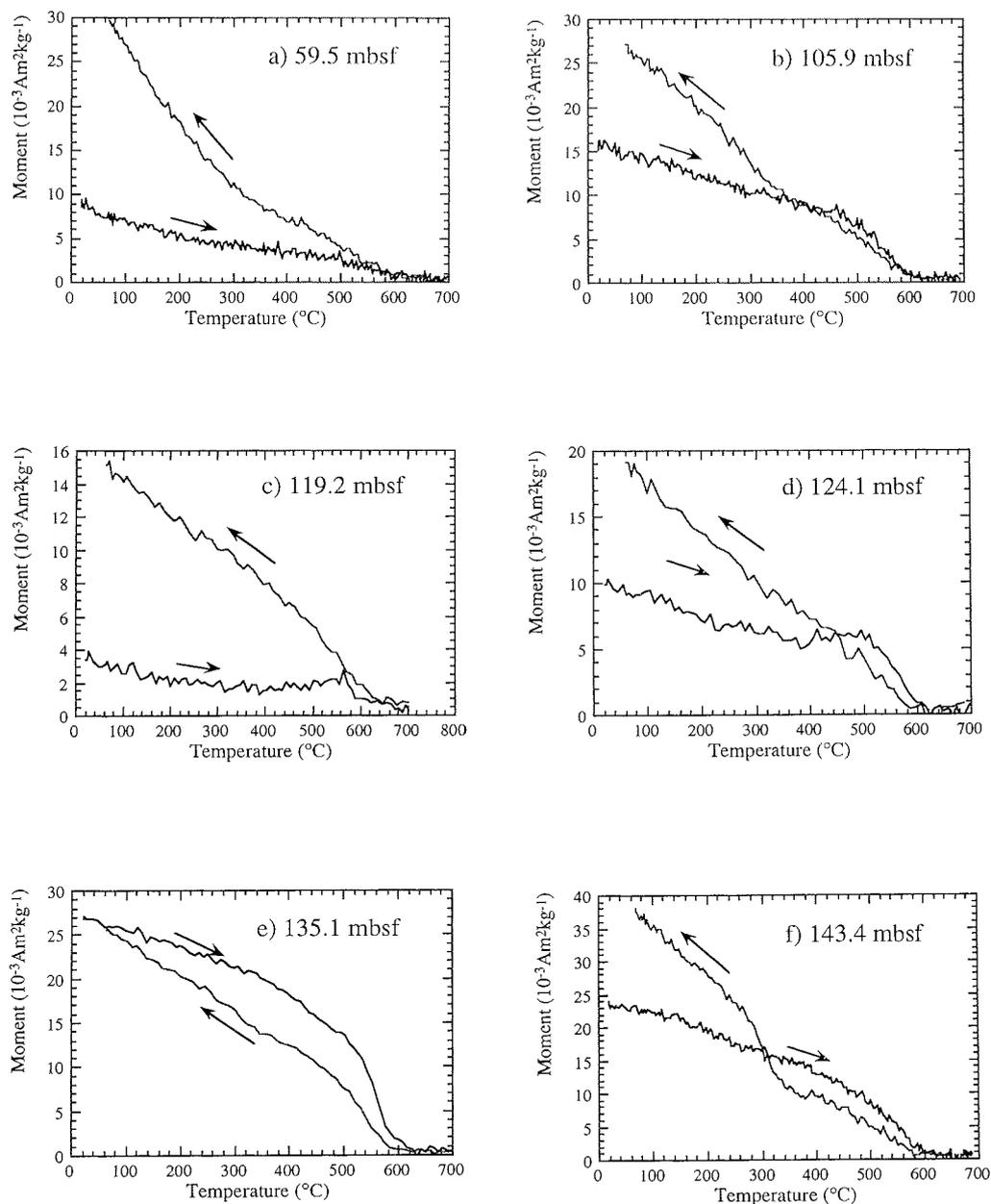
Fig. 4 - Variation of the magnetic moment vs. temperature in a heating-cooling cycle from room temperature to 700°C for samples from CRP-1 at depths of: a) 59.5 mbsf; b) 105.9 mbsf; c) 119.2 mbsf; d) 124.1 mbsf; e) 135.1 mbsf, and f) 143.4 mbsf. Though the paramagnetic component swamps the ferrimagnetic signal in many of the low magnetic intensity samples (a, c), a distinct Curie temperature at c. 580°C indicates that magnetite is the dominant magnetic mineral in the sequence.
