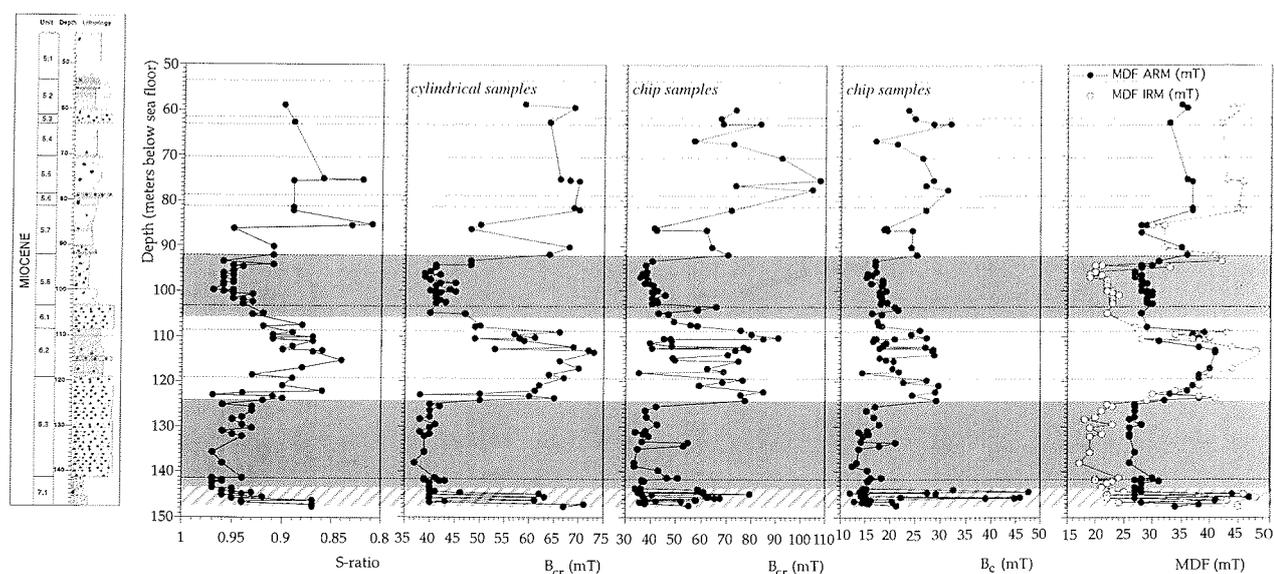
Fig. 2 - Downcore variation of the coercivity-dependent rock magnetic parameters (S-ratio,  $B_{cr}$  (from cylindrical samples),  $B_{cr}$  (from rock chips),  $B_c$  (from rock chips),  $MDF_{ARM}$  and  $MDF_{IRM}$ ) in the CRP-1 core. The zonation is the same as in figure 1 (see also Fig. 6).
