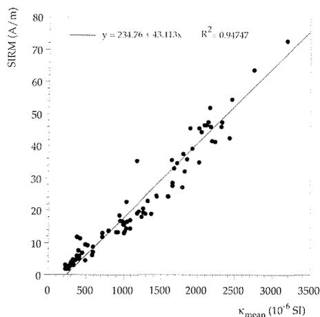
Fig. 7 - SIRM vs. low-field magnetic susceptibility ( $\kappa_{\text{mean}}$ ). The intersection of the regression line with the  $\kappa$ -axis provides an estimate of the base level contribution from the paramagnetic susceptibility (235  $\mu\text{SI}$ ).
