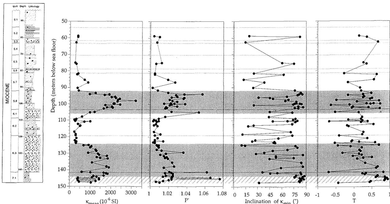
Fig. 6 - Downcore variation of the magnetic anisotropy parameters ( $\kappa_{mean}$ ,  $P'$ , Inclination of  $\kappa_{min}$  and  $T$ ) in the CRP-1 core. The corrected anisotropy degree  $P'$  and the shape factor  $T$  are from Jelinek (1981). The zonation is the same as in figure 1 (see also Fig. 2).
