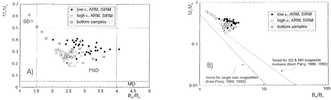
Fig. 5 - Plot of  $M_r/M_s$  vs.  $B_{cr}/B_c$  for samples from the CRP-1 core. "Bottom" samples refer to samples from below 143.8 mbsf. A) Plot with linear scales - the lines indicate the fields for single domain (SD), pseudo-single domain (PSD) and multidomain (MD) magnetites (cf. Day et al., 1977). B) Bilogarithmic plot - the trends for synthetic single size magnetites and magnetite mixtures (Parry, 1980, 1982) are shown for comparison.
