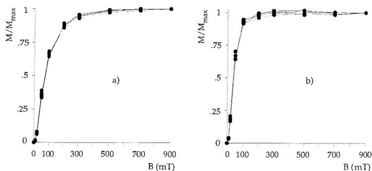
Fig. 3 - Representative IRM acquisition curves, up to 0.9 T, for: a) 7 samples from a high-coercivity interval (58 - 82 mbsf) which reach saturation at *c.* 500 mT, and b) 6 samples from a low-coercivity interval (97 - 100 mbsf) which reach saturation at *c.* 200 mT.
