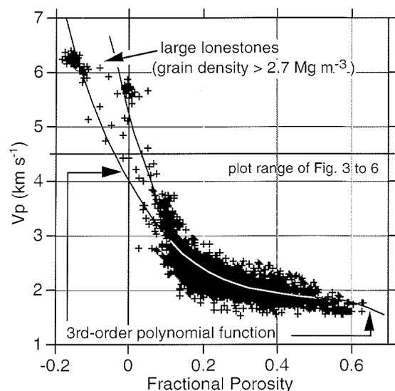
Fig. 1 - Comparison of P-wave velocity and porosity for all CRP-1 units, along with a 3rd-order polynomial fit.
