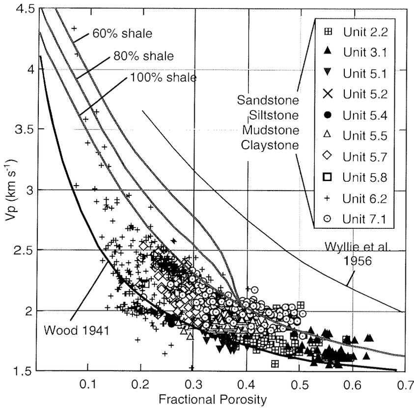
Fig. 5 - Comparison of P-wave velocity and porosity for the following CRP-1 lithologies: sandstone (Units 5.4, 6.2), sandstone dominant (Units 2.2, 3.1, 5.1, 5.5), siltstone dominant (Units 5.2, 5.7), mudstone (Unit 5.8) and claystone (Unit 7.1).
