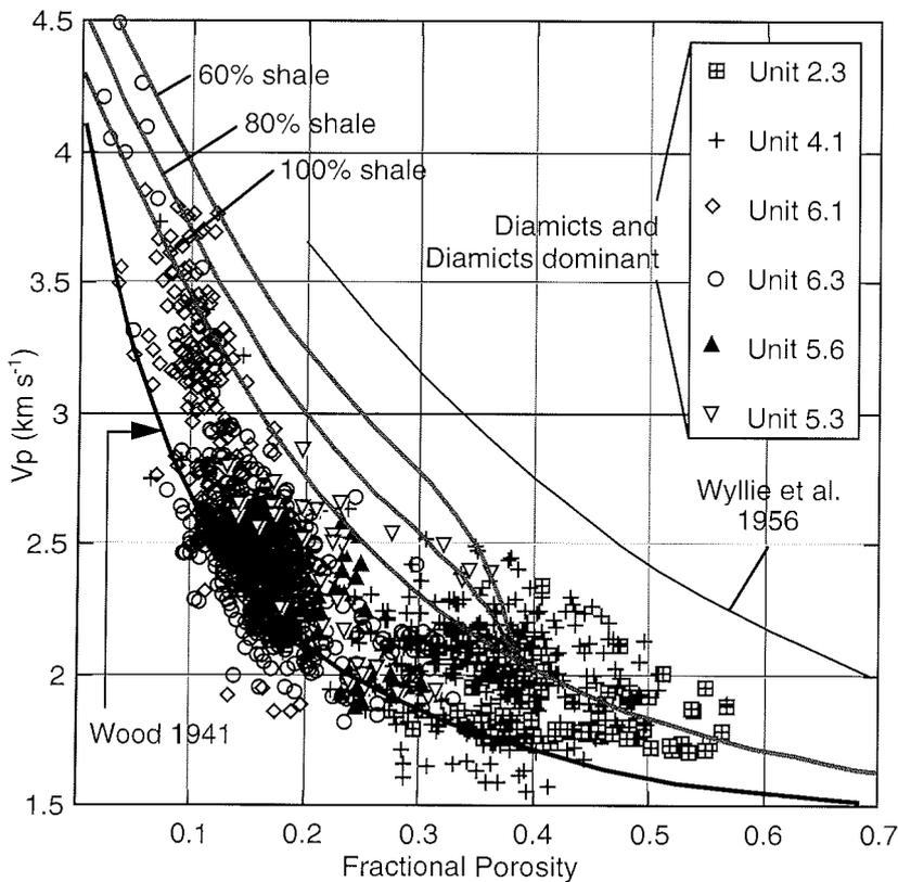
Fig. 6 - Comparison of P-wave velocity and porosity for the following CRP-1 lithologies: diamicts (Units 2.3, 4.1, 5.3, 6.1, 6.3) and diamicts dominant (Unit 5.6).
