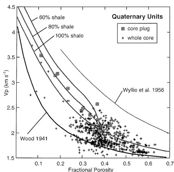
Fig. 3 - Comparison of P-wave velocity and porosity for all Quaternary CRP-1 units, for both whole-core and core-plug measurements. Model curves for suspensions (Wood, 1941), sandstone (Wyllie et al., 1956), and 60%, 80%, and 100% shale (Erickson & Jarrard, in press) are discussed in text.
