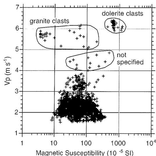
Fig. 2 - Comparison of P-wave velocity and magnetic susceptibility for all CRP-1 units.
