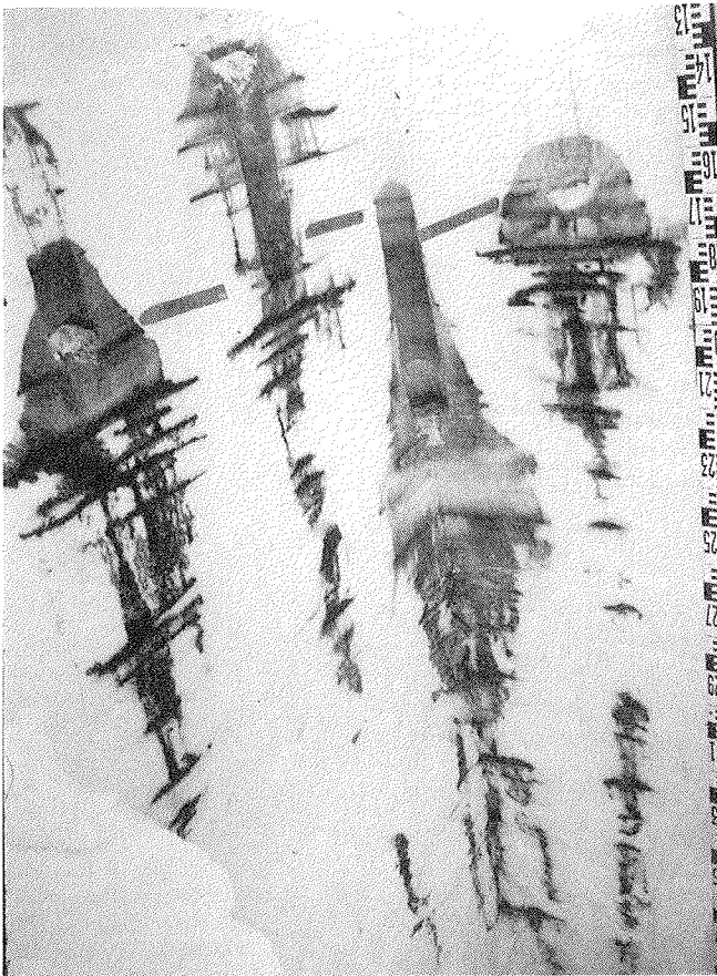
Fig. 1: Seepage path of dyed seawater filling in a dug-out borehole.
