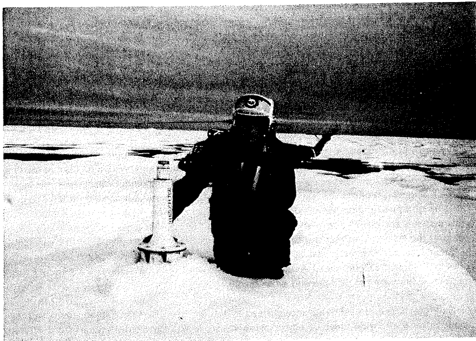
Fig. 2: Specially designed to be deployed on the ice, this buoy has been installed in a 1 m deep hole.
