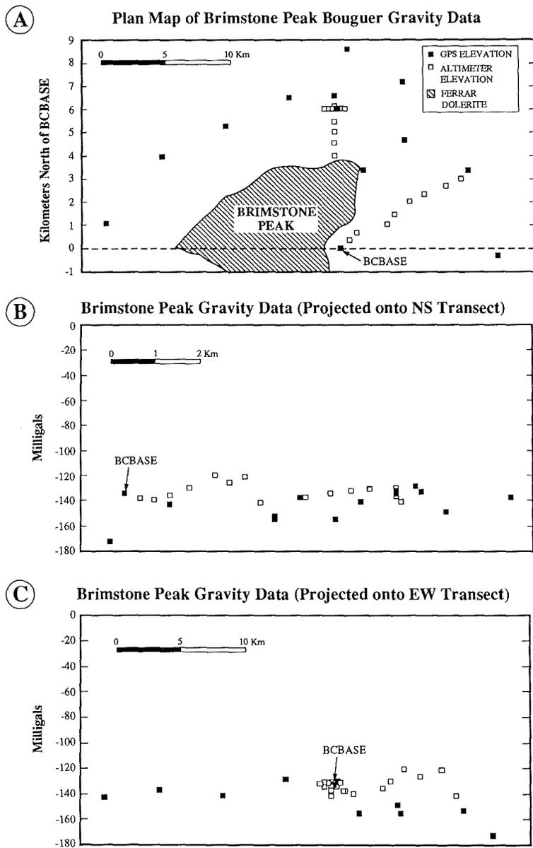
Fig. 2: Map showing Brimstone Peak local gravity survey (A) and gravity profiles of the gravity data projected onto NS and EW lines (B) and (C). Open symbols denote altimeter sites.
