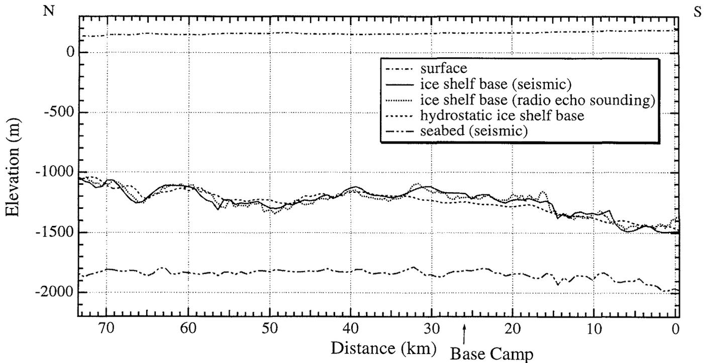
**Fig. 10:** Surface elevation from geodetic measurements, ice base determined from three different methods, and sea bed topography along the seismic profile in the area of the grounding line of the Foundation Ice Stream.
