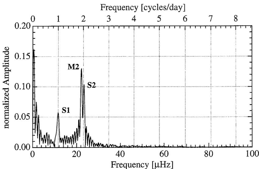
Fig. 5: Spectral analysis of the tidal record shown in Fig. 4.
