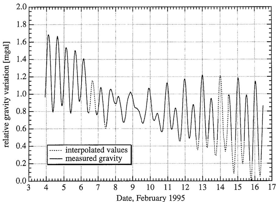
Fig. 4: Tidal record measured at the base camp on the Foundation Ice Stream.
