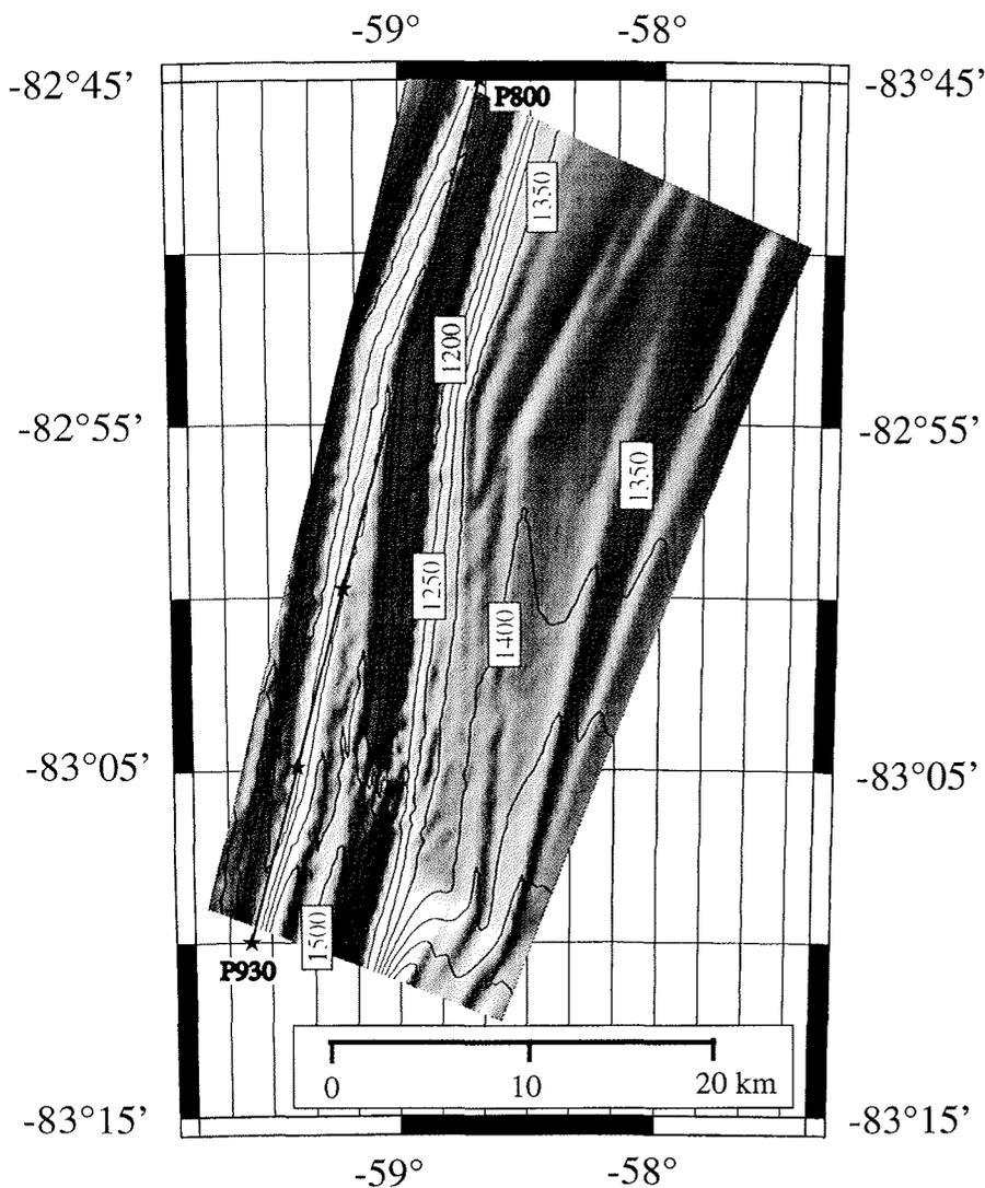
**Fig. 11:** Ice thickness distribution calculated from radio echo soundings. The contour interval is 50 m. The line marked with stars shows the position of the seismic profile from the base camp northwards.
