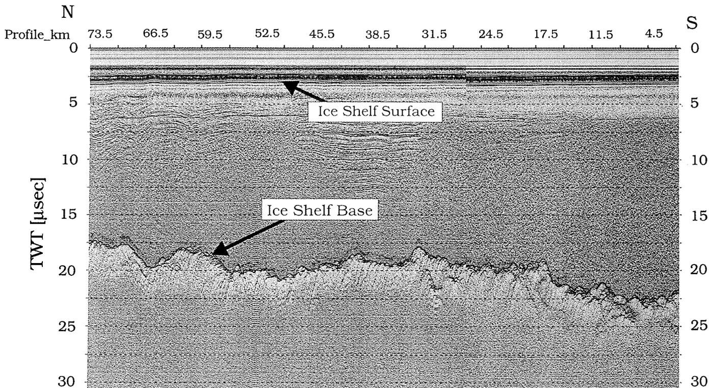
Fig. 8: Airborne radio echo sounding data profile 952002 directly adjacent to the seismic sounding, for the same section.
