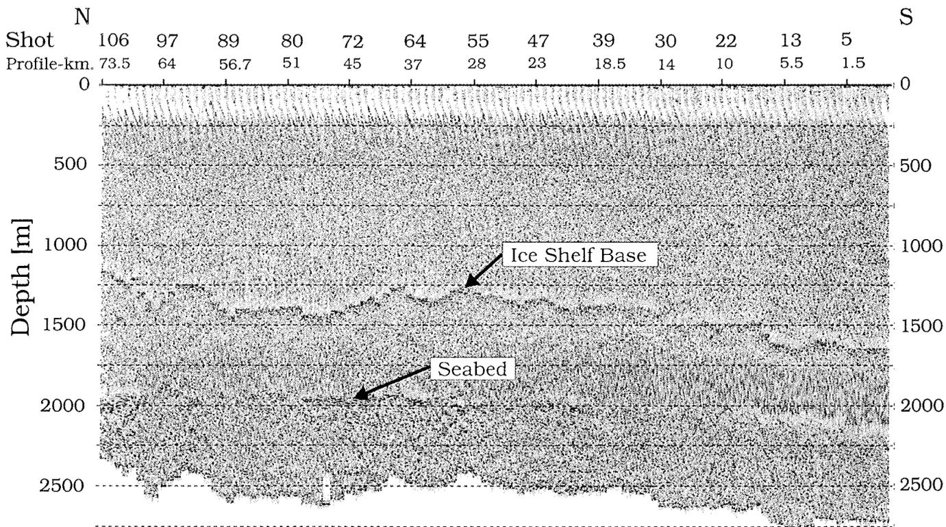
Fig. 7: Reflection seismic data of the grounding line area of the Foundation Ice Stream as depth section.
