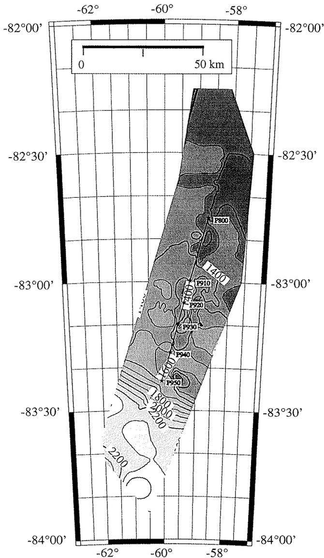
**Fig. 12:** The ice thickness within the transition zone of the Foundation Ice Stream from radio echo soundings, contours every 100 m. The line marks the position of the seismic profile.
