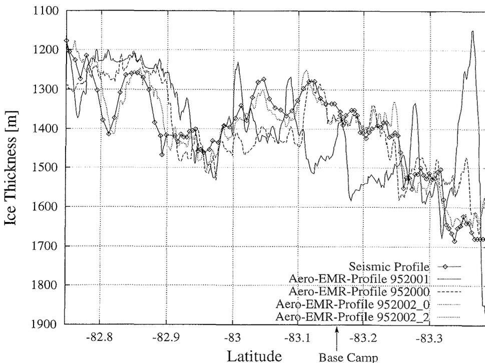
**Fig. 9:** Comparison of the ice thickness data in the grounding line area of the Foundation Ice Stream resulting from the seismic measurements and the airborne radio echo soundings.
