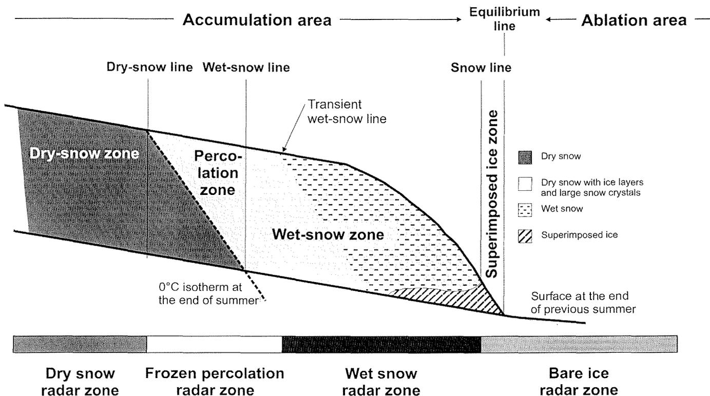
Fig. 2: Glacier snow zones and the corresponding radar glacier zones (after PATERSON 1994).
