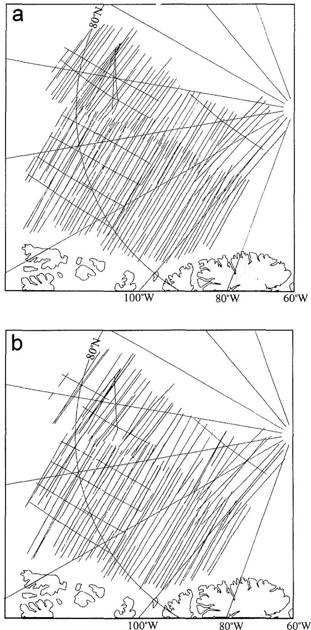
Fig.2: Russian tracklines before (a) and after (b) navigational corrections.
