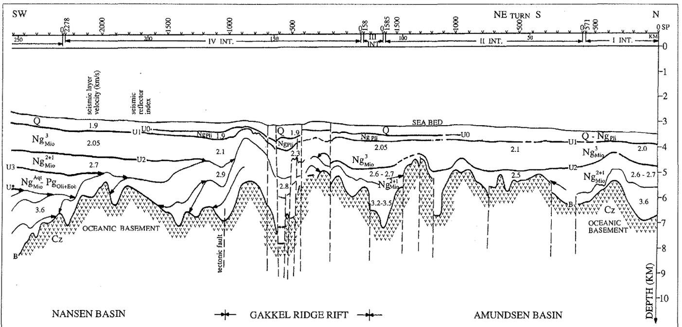
Fig. 5: Fragment of the seismic line 90701. Depth section. According to the data acquisition the whole transect consists of five parts with shot point sequences: I INT, II INT, III INT, IV INT, V INT. On top the shot points (SP) and their numbers as well as the horizontal scale in kilometers. Seismic units according to Figure 3 are included as well as seismic velocities in km/s. Assumed stratigraphic ages based on these studies are indicated.
