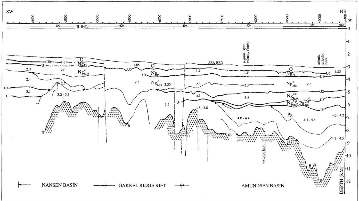
Fig. 6: Fragment of the seismic line 90702. Depth section. According to the data acquisition the whole transect consists of three parts with shot point sequences: I INT, II INT, III INT. On top the shot points (SP) and their numbers as well as the horizontal scale in kilometers. Seismic units according to Figure 3 are included as well as seismic velocities in km/s. Assumed stratigraphic ages based on these studies are indicated.
