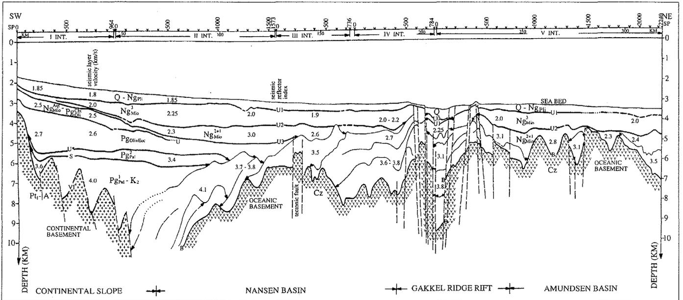
Fig. 4: Seismic line 90700. Depth section. According to the data acquisition the whole transect consists of five parts with shot point sequences: I INT, II INT, III INT, IV INT, V INT. On top the shot points (SP) and their numbers as well as the horizontal scale in kilometers. The seismic units accordingly to Figure 3 are included as well as their seismic velocities in km/s. Assumed stratigraphic ages based on these studies are indicated.
