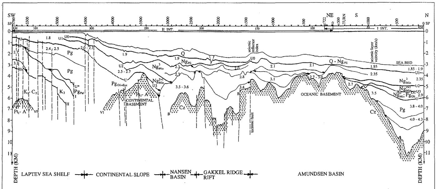
Fig. 7: Seismic line 90704. Depth section. According to the data acquisition the whole transect consists of two parts with shot point sequences: I INT, II INT. On top the shot points (SP) and their numbers as well as the horizontal scale in kilometers. Seismic units according to Figure 3 are included as well as seismic velocities in km/s. Assumed stratigraphic ages based on these studies are indicated.
