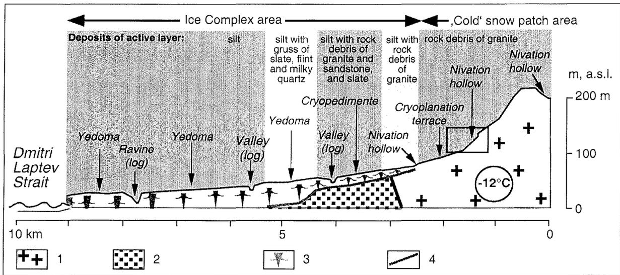
Fig. 3: Schematic profile of geocryological and geomorphological elements of Khaptagai Tas hills. 1: granite; 2: sandstone and slate; 3: Ice Complex; 4: lower boundary of the Ice Complex.
