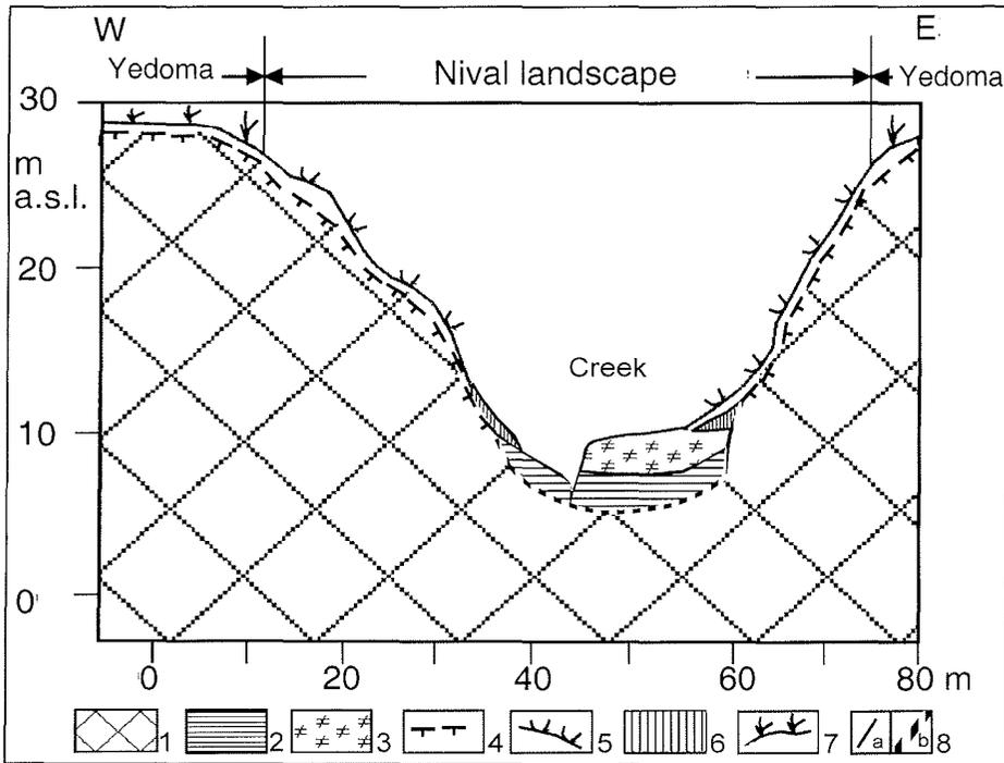
**Fig. 7:** Schematic profile of the „cold“ snow patch No. 1 (ravine type) and the surrounding nival landscape at Bykovsky Peninsula. 1: Ice Complex; 2: stratified ice; 3: stratified firm; 4: boundary of the active layer; 5: silt with plant detritus from the surface of the active layer; 6: talus; 7: surface of the active layer with plant cover of Subarctic grass tundra; 8: lithologic boundaries: 8a: determined, 8b: supposed.
