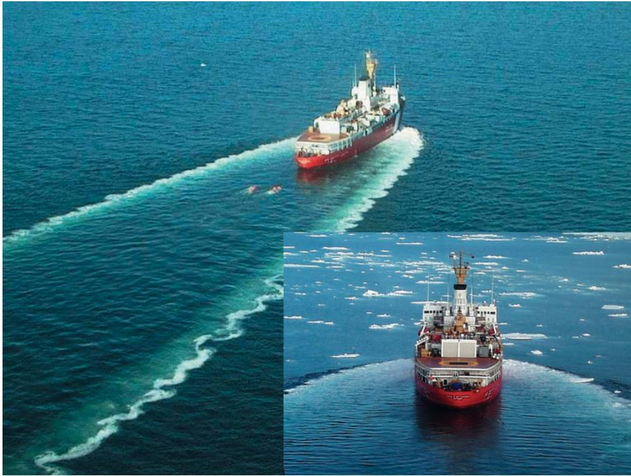
**Fig. 5:** The Canadian Coast Guard icebreaker “Louis S. St. Laurent” towing the seismic gear. Airguns are visible behind the ship. The bubble system designed to free the ship in dense ice, was successfully used to keep the wake free of small ice floes and growlers during streamer work.
