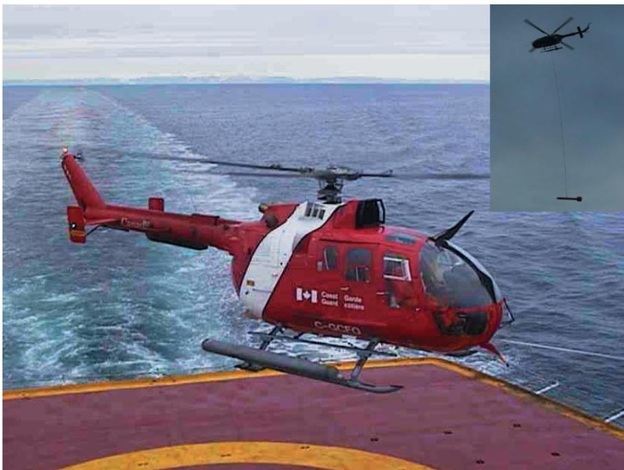
**Fig. 6:** Helicopter taking off for aeromagnetic survey flight (inset with bird) from the helideck of the CCG “Louis S. St. Laurent”.
