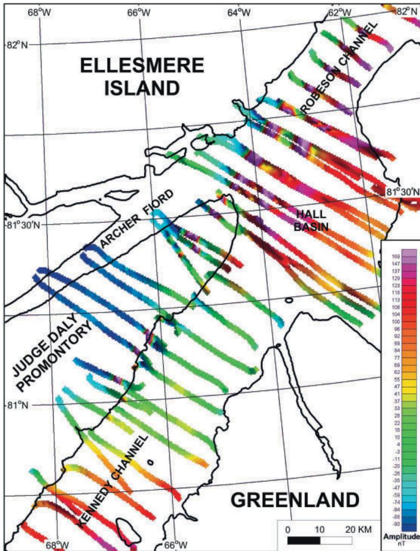
Fig. 2: Aeromagnetic survey lines collected during the 1982-1983 surveys over Robeson Channel, Hall Basin, Kennedy Channel (HOOD et al. 1985). Magnetic anomalies are presented along the lines with an equal-area colour scale.
