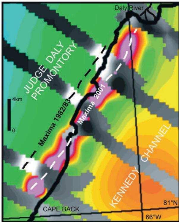
**Fig. 7:** Comparison of the positions of anomalies derived from the aeromagnetic survey Nares Strait 2001 (section taken from Fig. 5, without flight lines) with those of the 1982-1983 survey (taken from Fig. 1, but in grey scale: lighter grey refers to higher values of the magnetic anomaly field). The area shown here is the coastal strip between Cape Back and the mouth of the Daly River.
