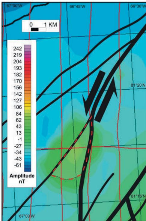
**Fig. 10:** Magnetic anomalies and position of the “Triangle” Tertiary basin. Survey lines shown in red. Outline of Tertiary basin (in dashed red) taken from TESSENSOHN et al. (in press). Fault structures simplified after VON GOSEN et al. (in press).
