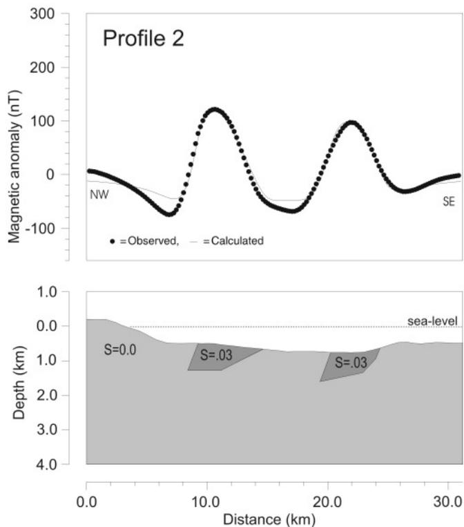
**Fig. 12:** Profile P2 across the main linear anomaly (frontal anomaly) in the Hall Basin – Robeson Channel and the anomaly running approximately parallel (parallel anomaly) in Hall Basin (see Fig. 5). Susceptibility  $S$  is given in SI-units.
