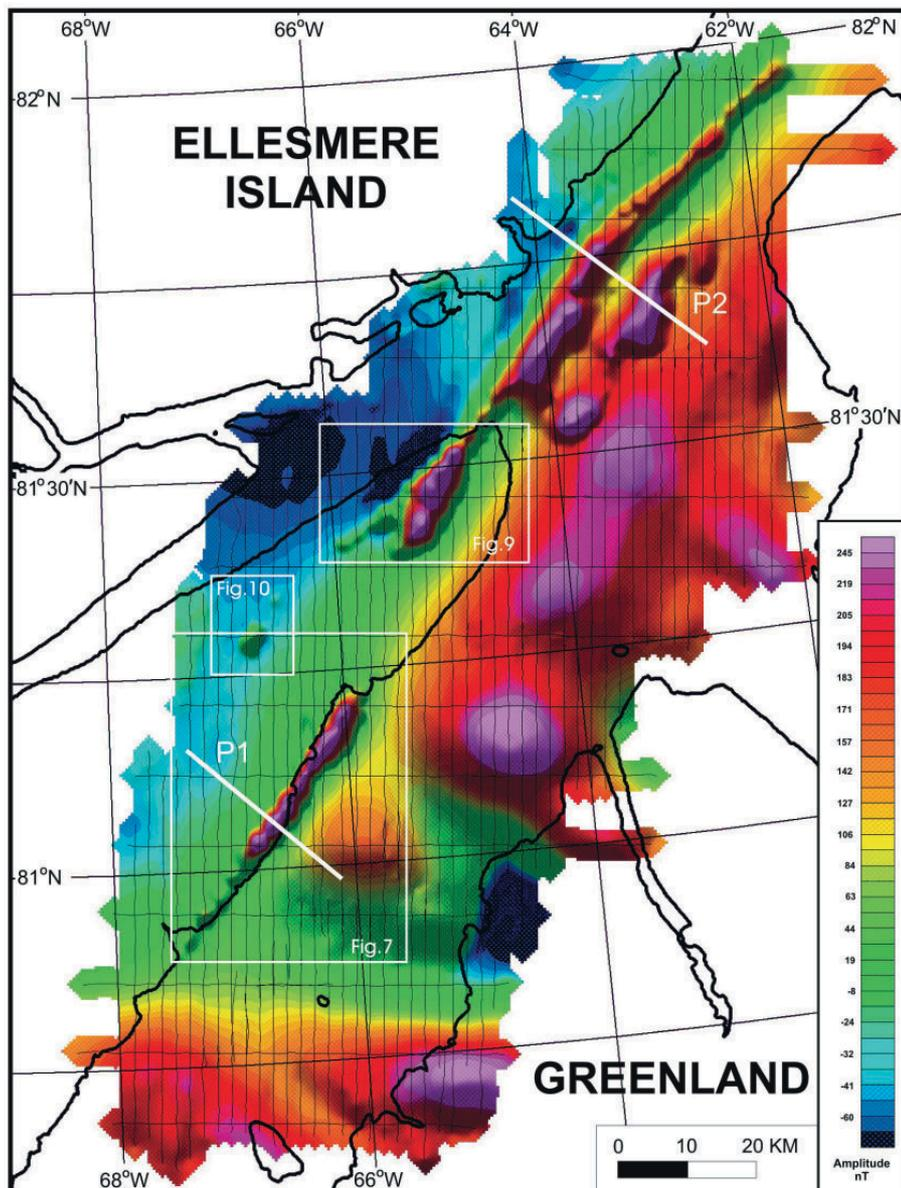
**Fig. 5:** Anomalies of the Total Magnetic Field over Hall Basin, Judge Daly Promontory, and Kennedy Channel. Colour scale is equal-area and shadowing direction is from 345°. Survey lines (in black) are displayed. P1 and P2 indicate the positions of the two synthetic profile lines extracted from the grid and modelled in Figure 8 (P1) and Figure 12 (P2). Locations of Figures 7, 9 and 10 are indicated (white boxes).
