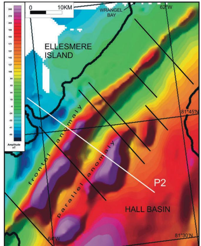
**Fig. 11:** Magnetic anomalies in Hall Basin and Robeson Channel. NW-SE orientated black lines indicate inferred faults. Colour scale and shadowing as in Figure 13.
