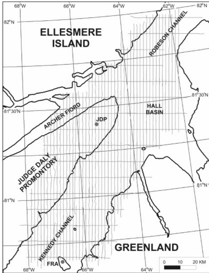
**Fig. 3:** Aeromagnetic survey lines and tie lines collected during the Nares Strait 2001 cruise. Base stations (grey dots) were installed on Franklin Island (FRA) and Judge Daly Promontory (JDP) to monitor diurnal variations of the magnetic field.
