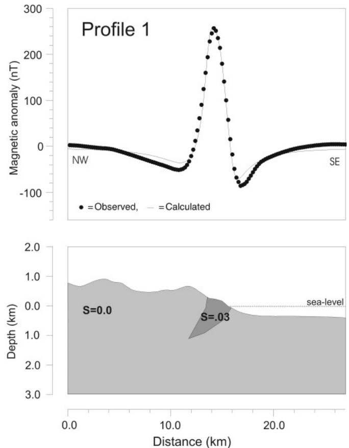
**Fig. 8:** Modelling a typical profile (P1) across the Tertiary basin along Kennedy Channel northeast of Carl Ritter Bay (position of profile, see Fig. 5). Susceptibility  $S$  is given in SI-units.
