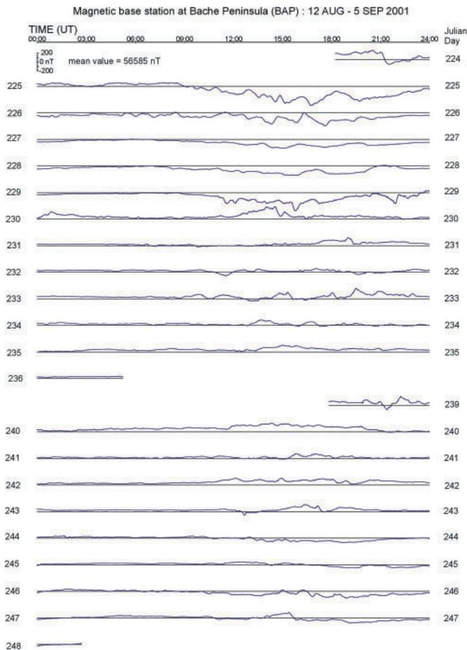
**Fig. 6:** Diurnal variations used for 2001 survey from Bache Peninsula (BAP). Survey flights were operated between 00:00 UT (Universal Time) and 08:00 UT to minimize the effect of the diurnal variation.
