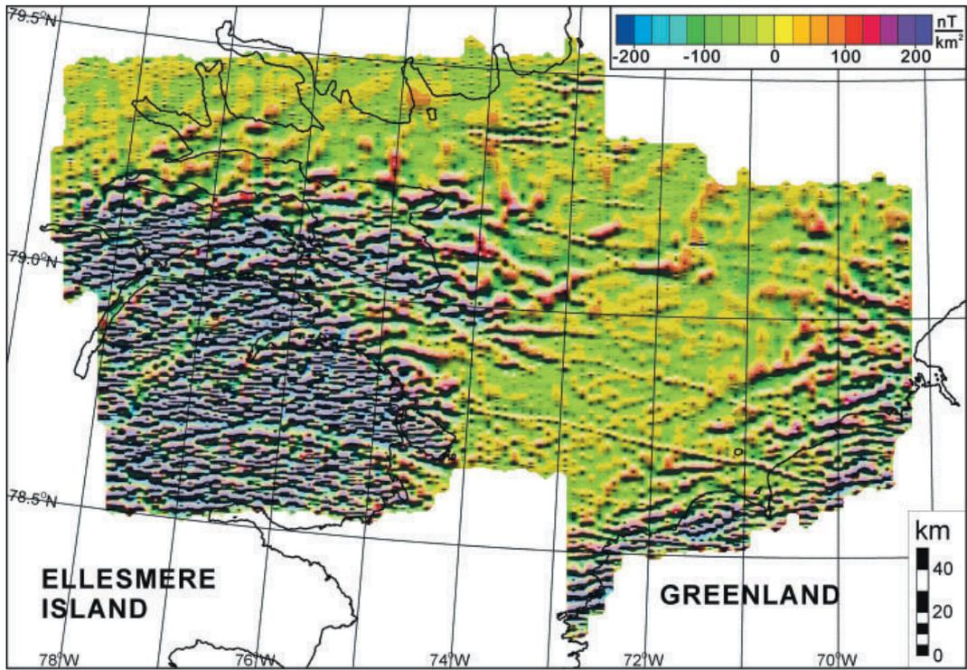
**Fig. 10:** Shadow illuminated 2<sup>nd</sup> vertical derivative map across Kane Basin between Greenland and Ellesmere Island. The high frequency component of the magnetic field resulting from shallow source-bodies are identified. Illumination is from the north.
