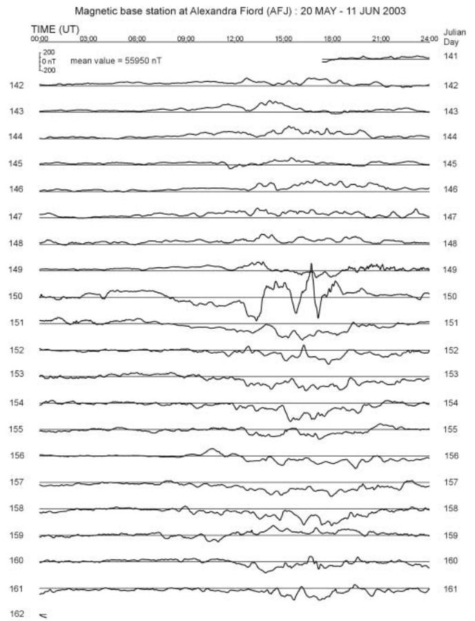
**Fig. 7:** Diurnal variations used for 2003 survey from Alexandra Fiord (AFJ). Survey flights were operated between 00:00 UT (Universal Time) and 08:00 UT to minimize the effect of the diurnal variation.
