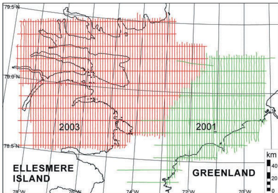
**Fig. 5:** Survey geometry of the 2001 and 2003 aeromagnetic surveys. A 2 km survey line spacing was designed on a Lambert conformal base (central meridian: 70 °W; standard parallels: 76°45' N and 79°15' N). Tie lines are spaced at 10 km.
