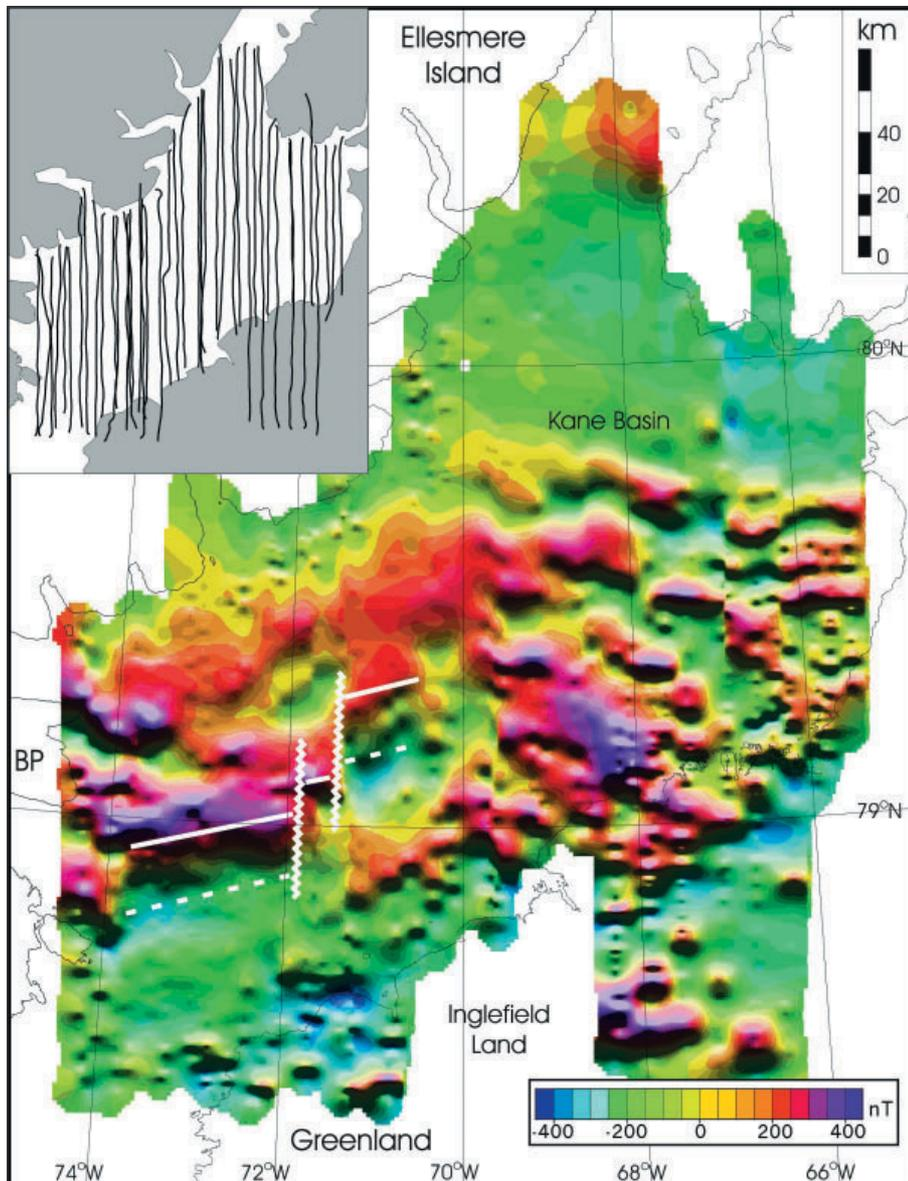
**Fig. 2:** Aeromagnetic data acquired in 1981 and 1982 between Inglefield Land and Ellesmere Island over Kane Basin (HOOD et al. 1985) with the interpreted offshore continuation of basement structures from Bache Peninsula (BP) (solid and dashed white lines) and the structural offsets (jagged white lines) defining the supposed 25 km of offsets along the Wegener Fault. The insert shows the location of the flight lines.
