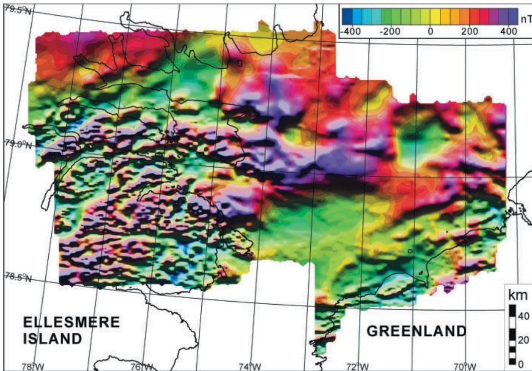
**Fig. 8:** Shadow illuminated total field anomaly map of the new survey data. Sun illumination angle is from the north. Generally, complex patterns of high amplitude - high frequency anomalies are observed onshore and near-shore; longer wavelengths within Kane Basin.
