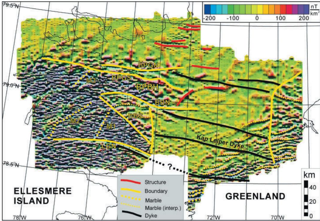
**Fig. 11:** Shadow illuminated 2<sup>nd</sup> vertical derivative map with interpretive overlay. Shown are the correlations with onshore marble belts (M1, M2, M3); Kap Leiper Dyke; inferred offshore dykes; inferred marble belts and interpreted structures; LGN = Leffert Glacier northern edge; BPGN = Bache Peninsula graben north; BPGS = Bache Peninsula graben south; BPGH = Bache Peninsula basement high; BBN = Buchanan Bay northern shore; BBS = Buchanan Bay southern shore.
