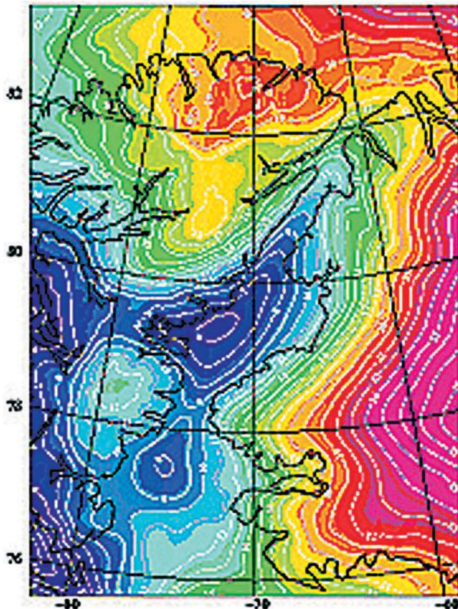
Fig. 8: Geoid heights (meter) in the Nares Strait region from the ArcGP geoid model. Crosses show location of GPS sea-level points.
