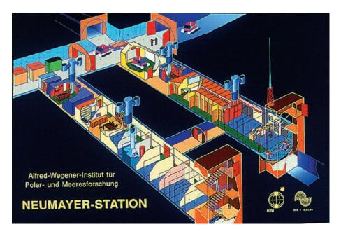
**Fig. 12:** Schematic diagram of Neumayer Station II (NM-II) showing the station design below the ice (not showing the vehicle garage), (D. Enss / Polarmar)
