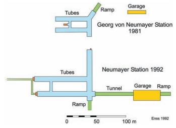
**Fig. 10:** Schematic diagram showing proportions of the two stations Georg von Neumayer (GvN) constructed in 1981 and its successor Neumayer Station II (NM-II) constructed in 1992 (D. Enss / Polarmar).
