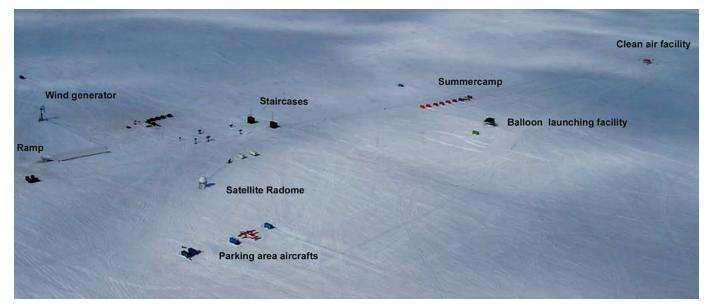
Fig. 11: Research station Neumayer II (NM-II) in 1999. Aerial view of the station in total including the remote clean air observatory. The ramp and the staircases mark the outline of the station beneath the snow surface (D. Steinhage).
