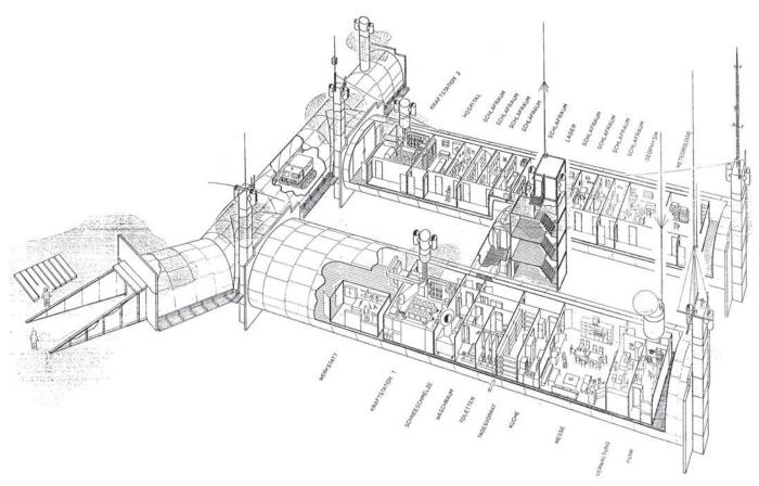
Fig. 1: Georg von Neumayer Station (GvN). Schematic diagram of the tube construction situated beneath the snow surface (Figure D. Enss / Polarmar).
