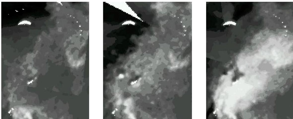
*Fig. 4.5: Quikscat Ku-band backscatter maps of September 28 (left), 29 (centre), and 30 (right), showing backscatter changes due to the passage of a region of warm air. Bright grey values indicate high backscatter.*
