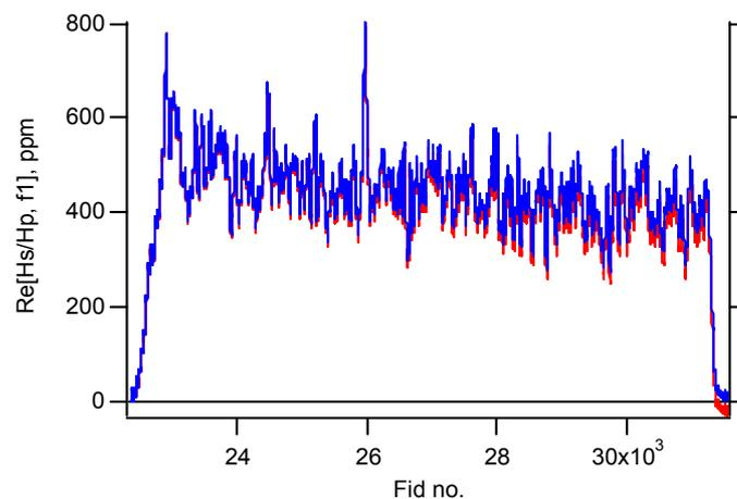
**Figure 4:** Typical profile of inphase component of  $f_1$  (3.6 kHz) showing original (red, stippled) and drift-corrected trace (blue, solid). February 23, 2<sup>nd</sup> flight, file 200302231204\*.
