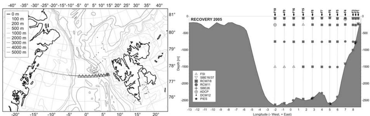
Fig. 3.1: Location of CTD stations and moorings (left) and distribution of instruments at the mooring array (right) recovered and redeployed in 2004.
