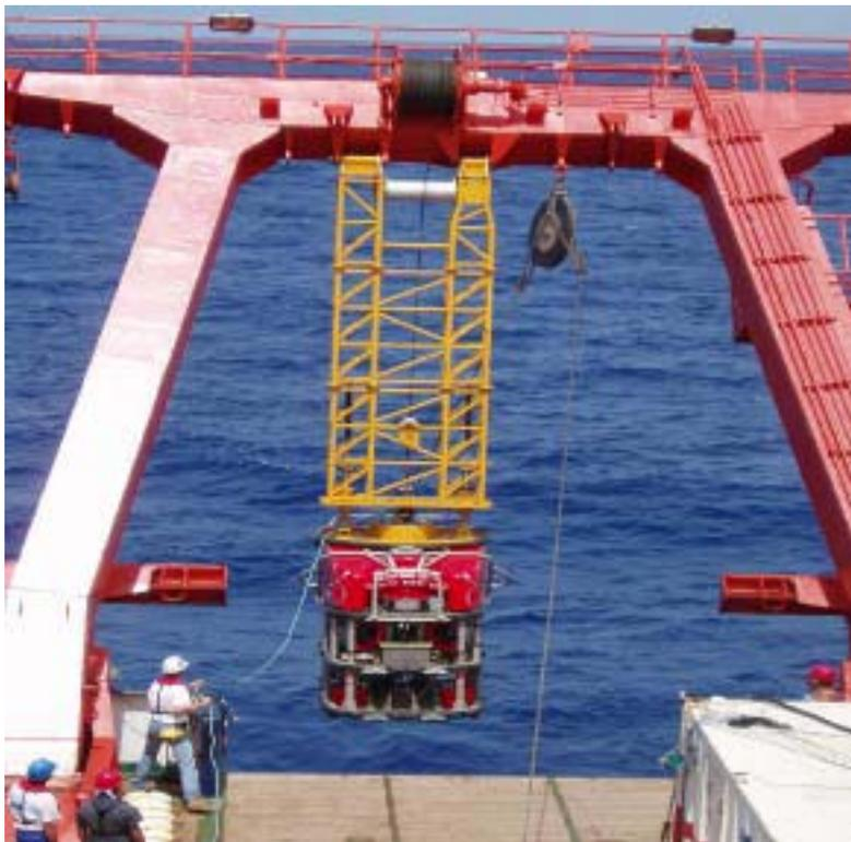
*Figure 5-14: Launching of the ROV with a new deployment frame.*
