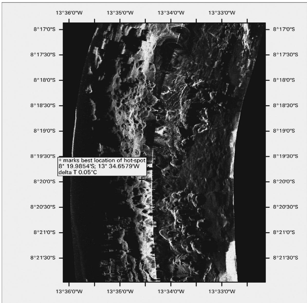
*Figure 5-10: Northern tip of Segment A2. The + marks the site of highest water temperature anomaly from the TOBI vehicle (“hotspot”), delta T = 0.05C, altitude 15m, bottom depth 2940m. Possible hydrothermal source, located on the crest of an axial volcanic ridge as it intersects an axial valley wall fault.*
