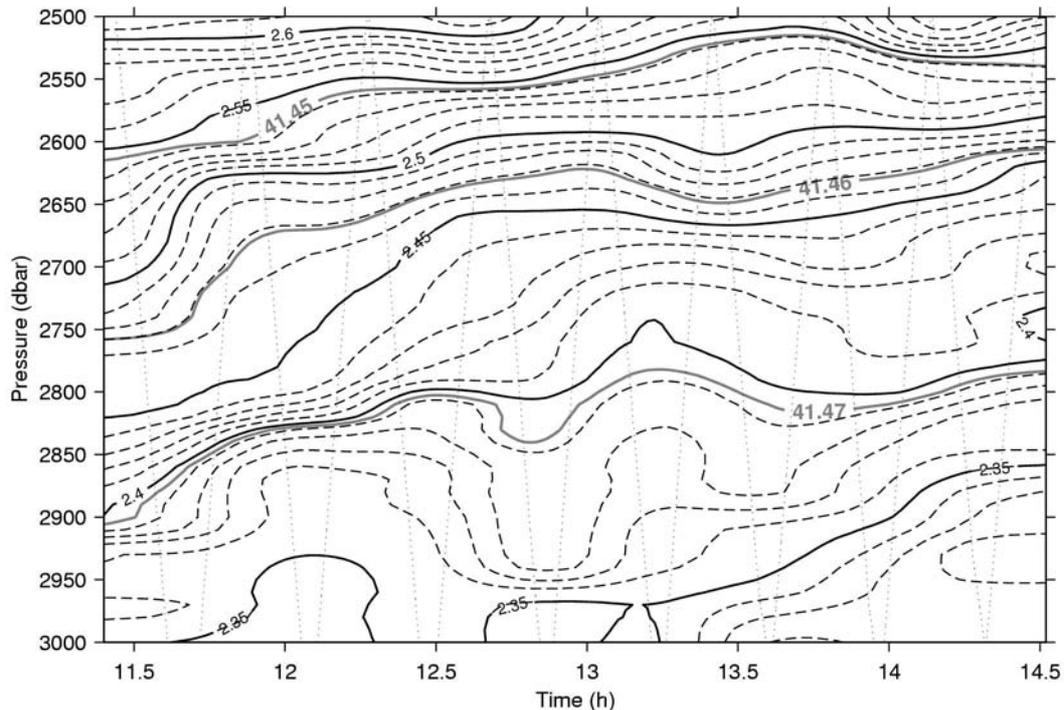
Figure 5-23: Temporal evolution of potential temperature in °C during the yoyo CTD cast 1287. Grey lines denote potential density relative to 3000 m ( $\sigma_3$ ) in  $\text{kg/m}^3$ .
