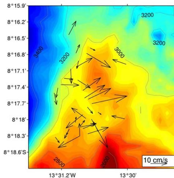
Figure 5-24: LADCP currents in the lowest depth bin above the seafloor.
