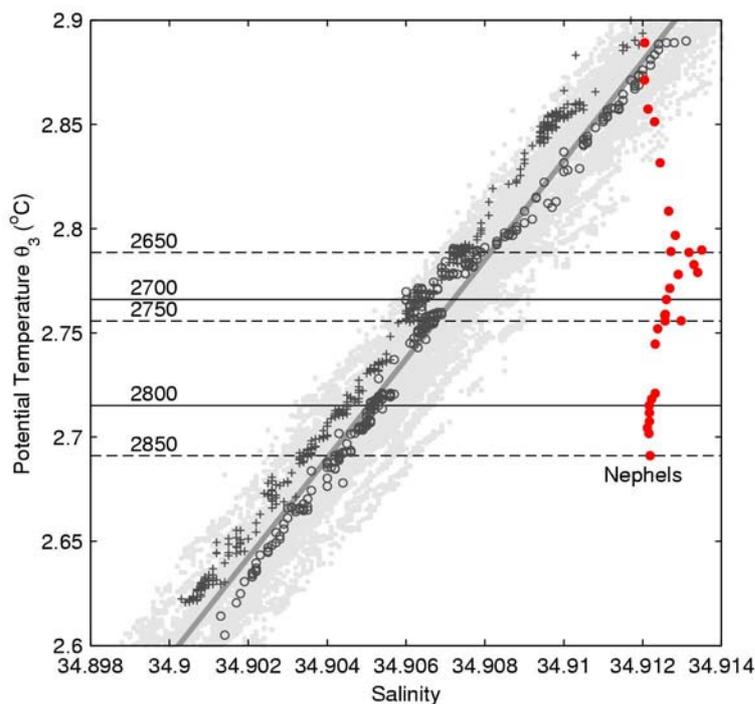
*Figure 5-22: Potential Temperature vs. Salinity diagram. Light gray: background of all CTD stations; medium gray line: average T-S relationship; dark gray circles: CTD profile 1230; dark gray crosses: CTD profile 1276. Added are depth lines and scaled nephels (MAPR) plotted against temperature.*
