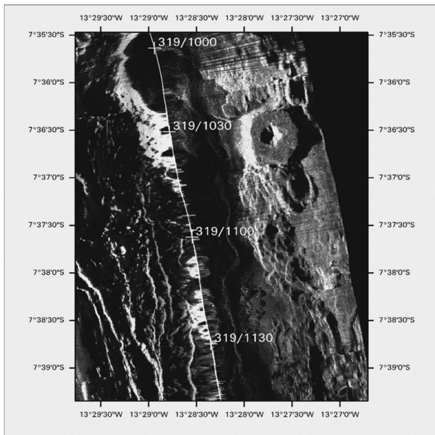
*Figure 5-3: Volcano 1, northern-end of Segment A1. The time stamp, along the vehicle track, refers to Julian day, hour and minute for the vehicle. Navigation is predicted position of the vehicle using inertial navigation that is referenced to ship's GPS position. Vehicle positioning is good to  $\pm 100m$ .*
