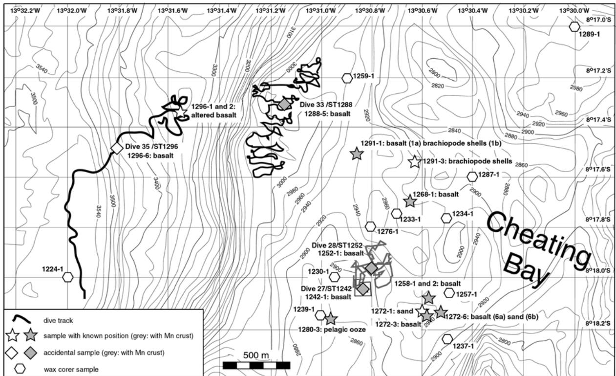
Figure 5-34: Location of seafloor samples obtained during M62-5b in the Cheating Bay area. Note that dive tracks are only shown when accidental samples were recovered.
