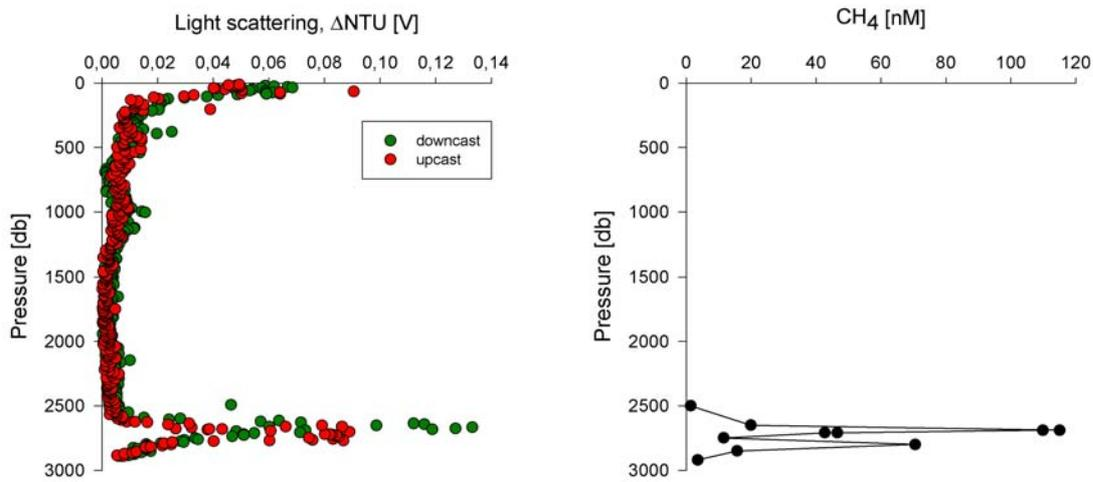
*Figure 5-26: Light backscattering and methane concentrations of station 1230.*
