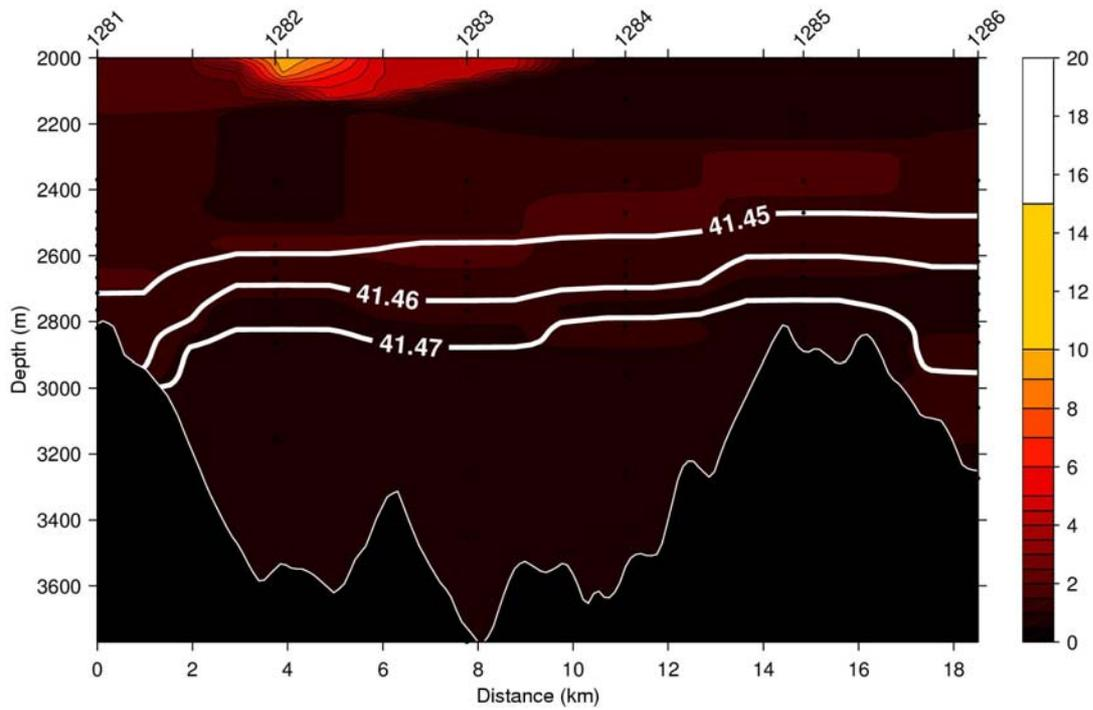
Figure 5-28: Section 1, CH<sub>4</sub> concentration [nM] and density [ $\sigma_3$ ]
