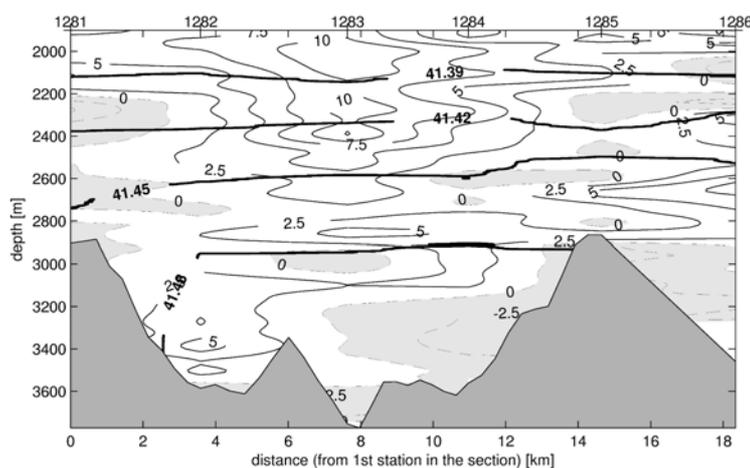
*Figure 5-25: LADCP velocities in the rift valley at 8°10' S below 2000m. Velocities are given in cm/s. Contour interval is 2.5cm/s. Southward velocities are shaded. Strong solid lines indicate  $\sigma_3$  contours. Profile numbers are given at the top.*
