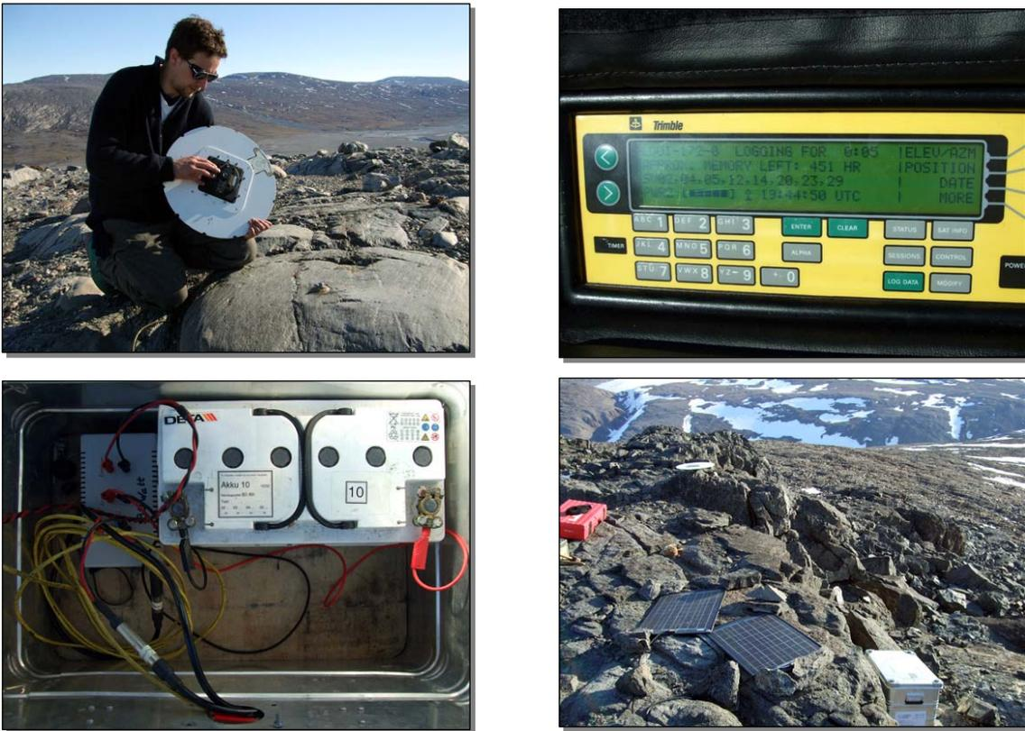
*Fig. 7.1: Typical set-up of a GPS station.*
