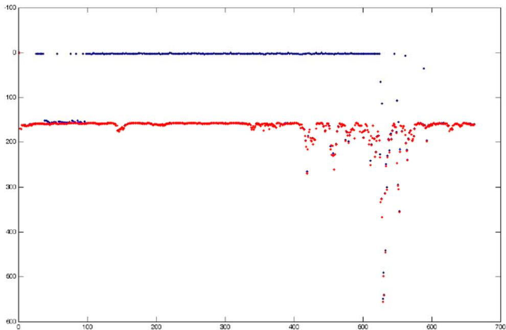
Fig. 3.3: First and last pressure of each CTD-logger record interval (duration 30 min every 12 h). Pressure is in dbar against CTD-logger record number
