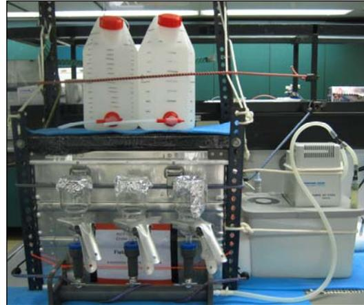
*Fig. 5.3: Filtration ramp for CTD water (left) and inline filter holder system (right) on board Polarstern during ARK-XXIII/1*
