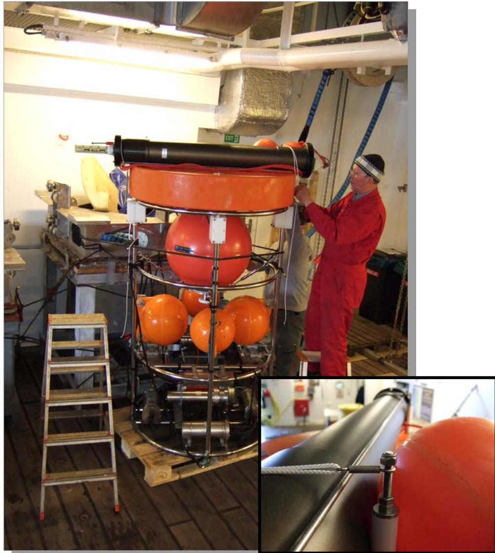
*Fig. 3.2: NGK Automated Elevator System with an added buoyancy slice of syntactic foam and the Optimare/Sea-Bird Electronics CTD-logger on top before deployment in 2007 (left). The CTD-logger is initially fixed to the winch frame utilizing corrosion links (bottom right).*
