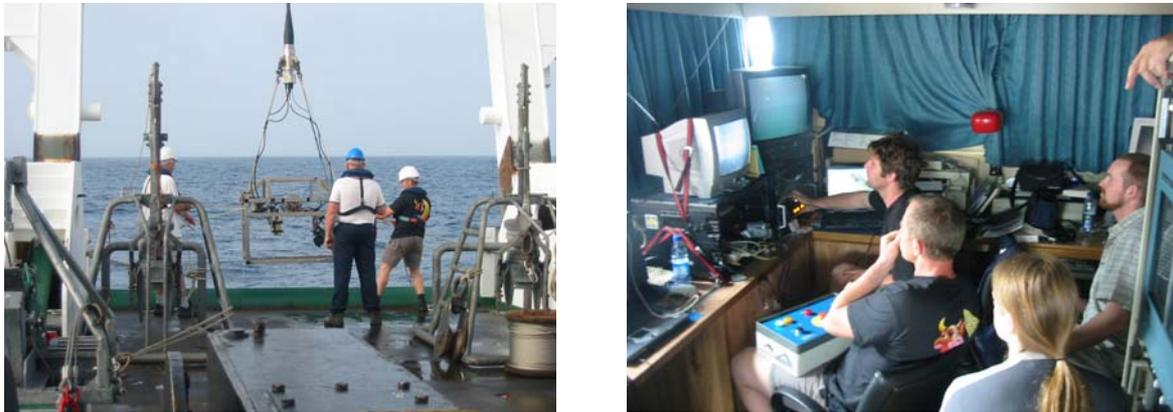
**Figure 16:** Video operations. On the left side, the video frame is launched with navigator camera on the left side and inspector camera on the right side. The picture on the right, shows the bridge configuration with the two camera displays, navigation computer, remote winch control and observers.
