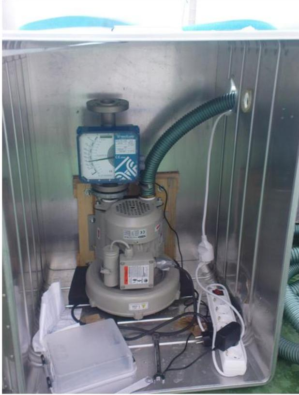
Picture 2.7.1 Pump and flow meter inside box.
