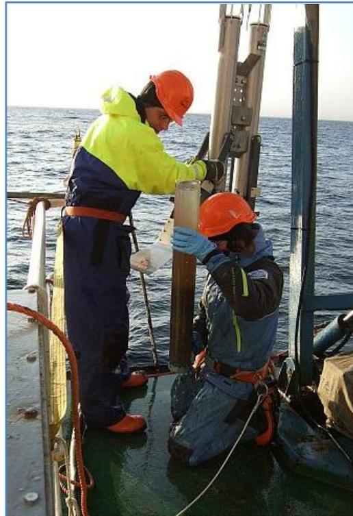
Within 12 to 48 hours after sampling, the cores were sliced into 1cm slices using an extruder (Oy Kart AB, Finland). A stainless steel spoon was used to transfer the 1cm slices into small containers (65 ml to 210 ml). The sediment containers were marked and frozen the same day at  $-18^{\circ}\text{C}$ . The cores were described during slicing. A PDF document with core lengths, descriptions, time between sampling and slicing, and planned analyses is available on request.
