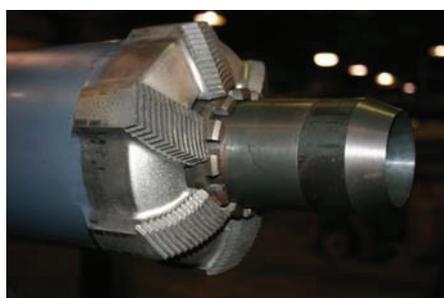
**Extended-Nose Corer** - As noted above the extended-nose corer is similar to IODP's XCB-type coring system. The non-rotating spring-loaded barrel is in advance of the
