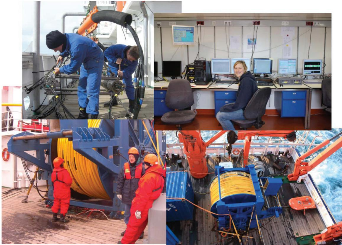
Fig. 5.2: SERCEL SEAL™ digital multichannel seismic system and the recordings units.
