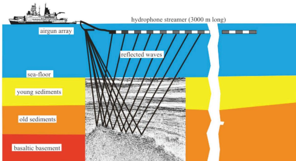
Fig. 5.1: Principle of marine seismic reflection surveying.
