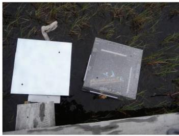
Figure 5-1 Sampling spots in a waterlogged polygon centre covered by a transparent (right) and an opaque (left) chamber.
