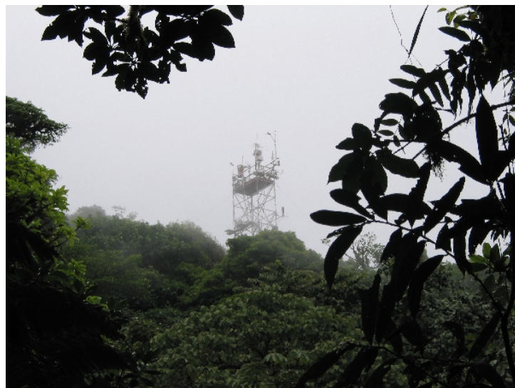
Figure 2.1: Meteorological tower (24 m height) with our measurement equipment on top.
