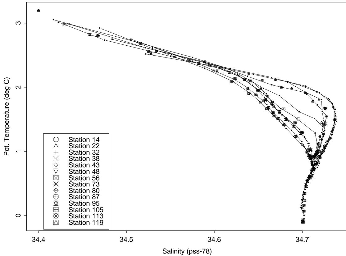
**Figure 3:** Theta-salinity for all of the large volume cast data with a QC flag of 2 for both temperature and salinity. CTD theta values with Rosette bottle salinities (small filled squares) are overlain for comparison.
