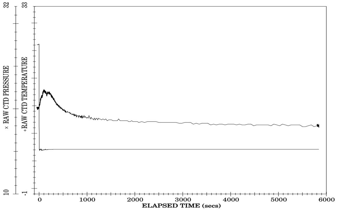
Figure 2a: CTD #1 Warm-to-Cold Thermal Shock Data
