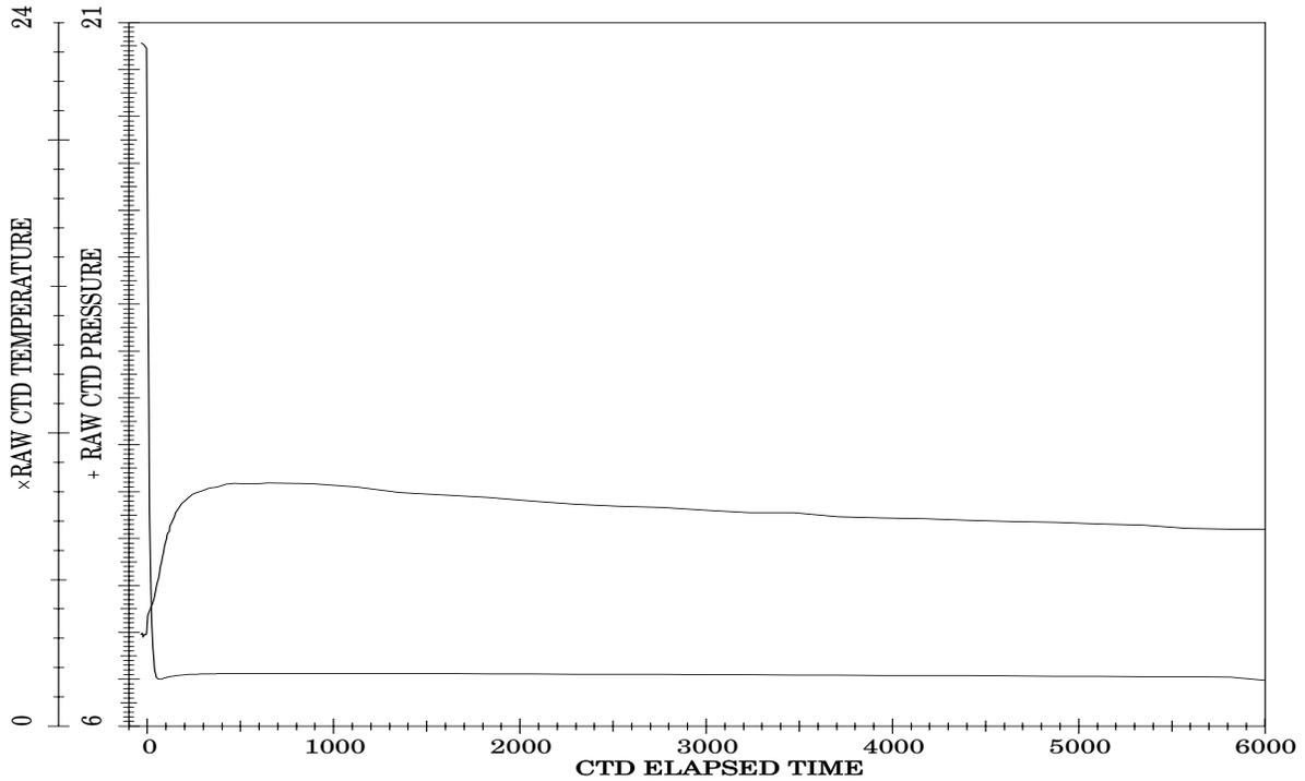
Figure 4: CTD #2 Warm-to-Cold Thermal Shock Data
