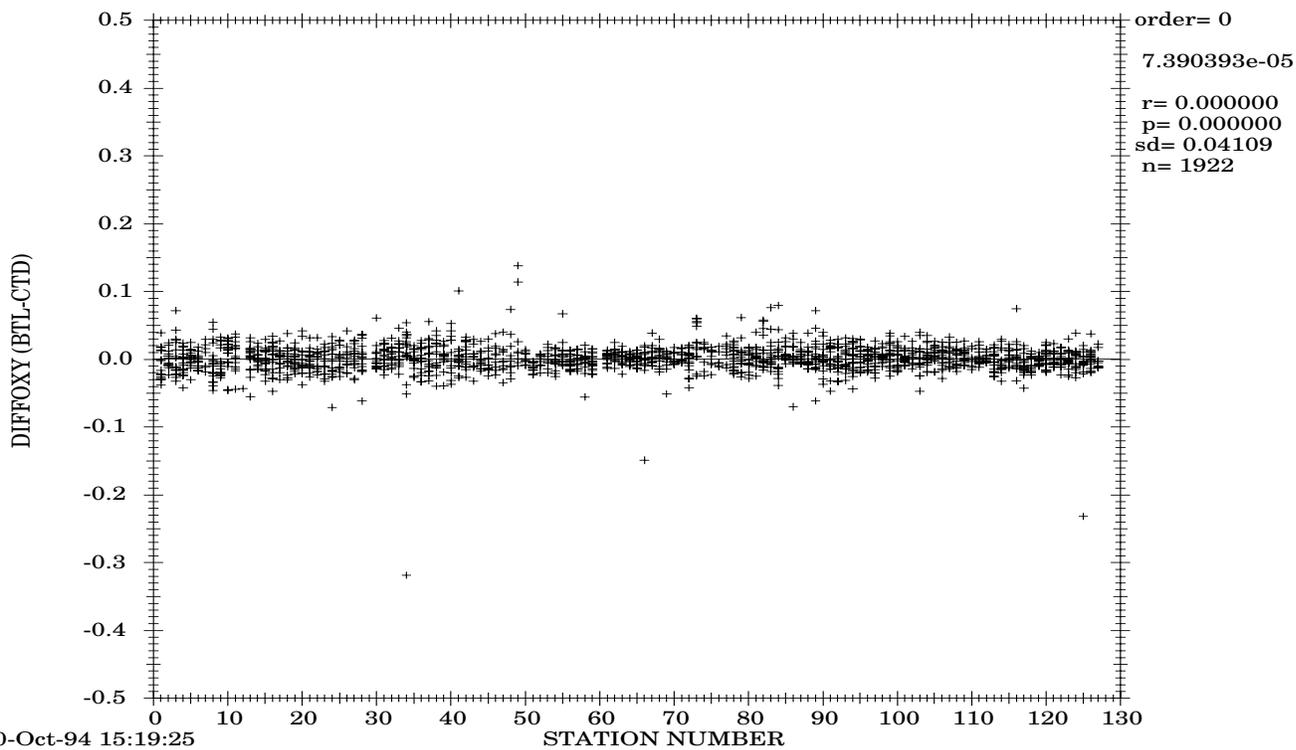
Figure 9b: JUNO1 Residual Diss.Oxygen UpBottle-DownCTD Differences - Prs>1500dbar
