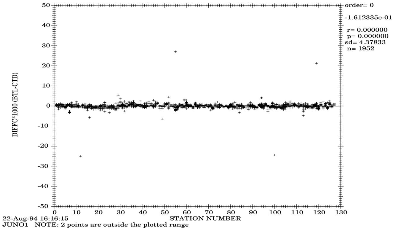
Figure 8b: JUNO1 Residual Conductivity Bottle-CTD Differences - Prs>1500dbar
