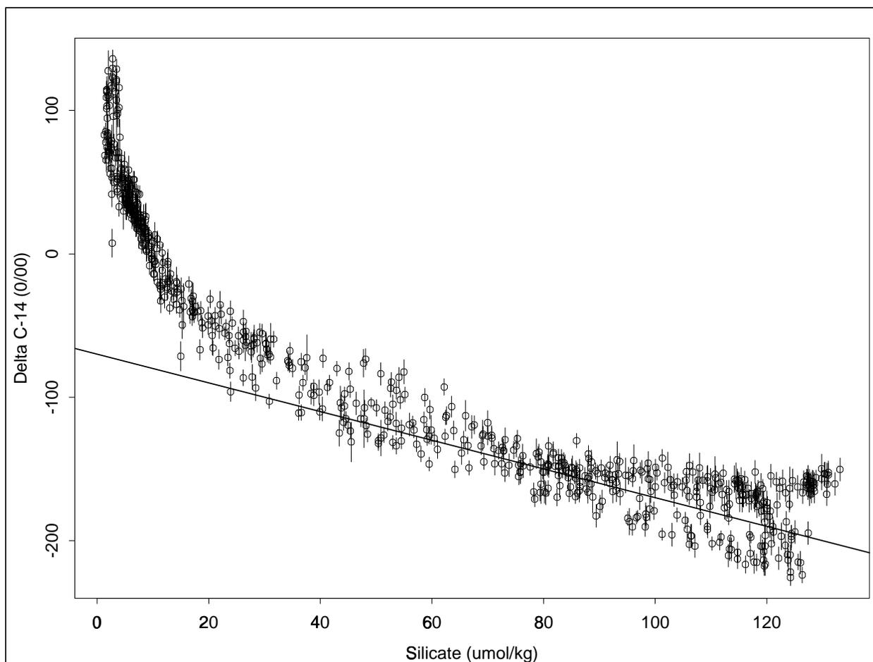
**Figure 3:**  $\Delta^{14}\text{C}$  as a function of silicate for P116A17A AMS samples. The straight line shows the relationship proposed by Broecker, *et al.*, 1995 ( $\Delta^{14}\text{C} = -70 - \text{Si}$  with radiocarbon in ‰ and silicate in  $\mu\text{mol/kg}$ ).
