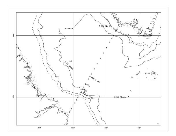
Figure 2: Mooring plan for Hudson 96026. Mooring locations marked by  $\Delta$ 's; +'s mark the positions of CTD / rosette stations along WOCE repeat section AR7W, the centre section of the five planned sections on figure 1. Moorings SS North, SS West and L are on the second CTD section, SS South is on section 4 and SS East is on section 5.
