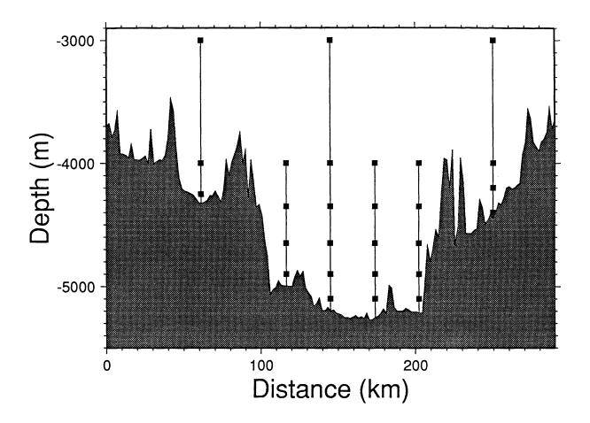
Figure 3. The mooring array in the Samoan Passage and underway bathymetry. The perspective is looking northward, so mooring 1 is on the left and mooring 6 is on the right. The squares indicate the locations of current meters.
