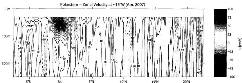
Fig. 2: Zonal current velocity along a meridional section at 15° to 20°W during *Polarstern* cruise ANT-XXIII/10 in April 2007. Most prominent is the equatorial current system with the Equatorial Undercurrent (EUC) at 50 m depth at the equator (up to 1 m/s) and the South Equatorial Undercurrent (SEUC) at 100 to 200 m depth at 5°S (up to 0.4 m/s). Further north there are several eastward and westward current bands mainly associated with the enhanced eddy field in the region.
