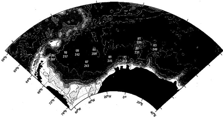
Fig. 9.1: Sound source array as currently installed. Numbers next to the dots indicate sound source labels and corresponding mooring numbers. Mooring 240 / sound source W3 will be recovered and redeployed during ANT-XXV/2.
