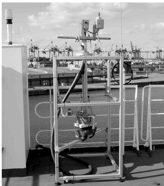
*Fig. 3: The on-deck instrumentation of the MAX-DOAS instrument. The telescope unit is mounted on a cardanic system whereby the brush is used for braking the movement influenced by the ship's movement.*
