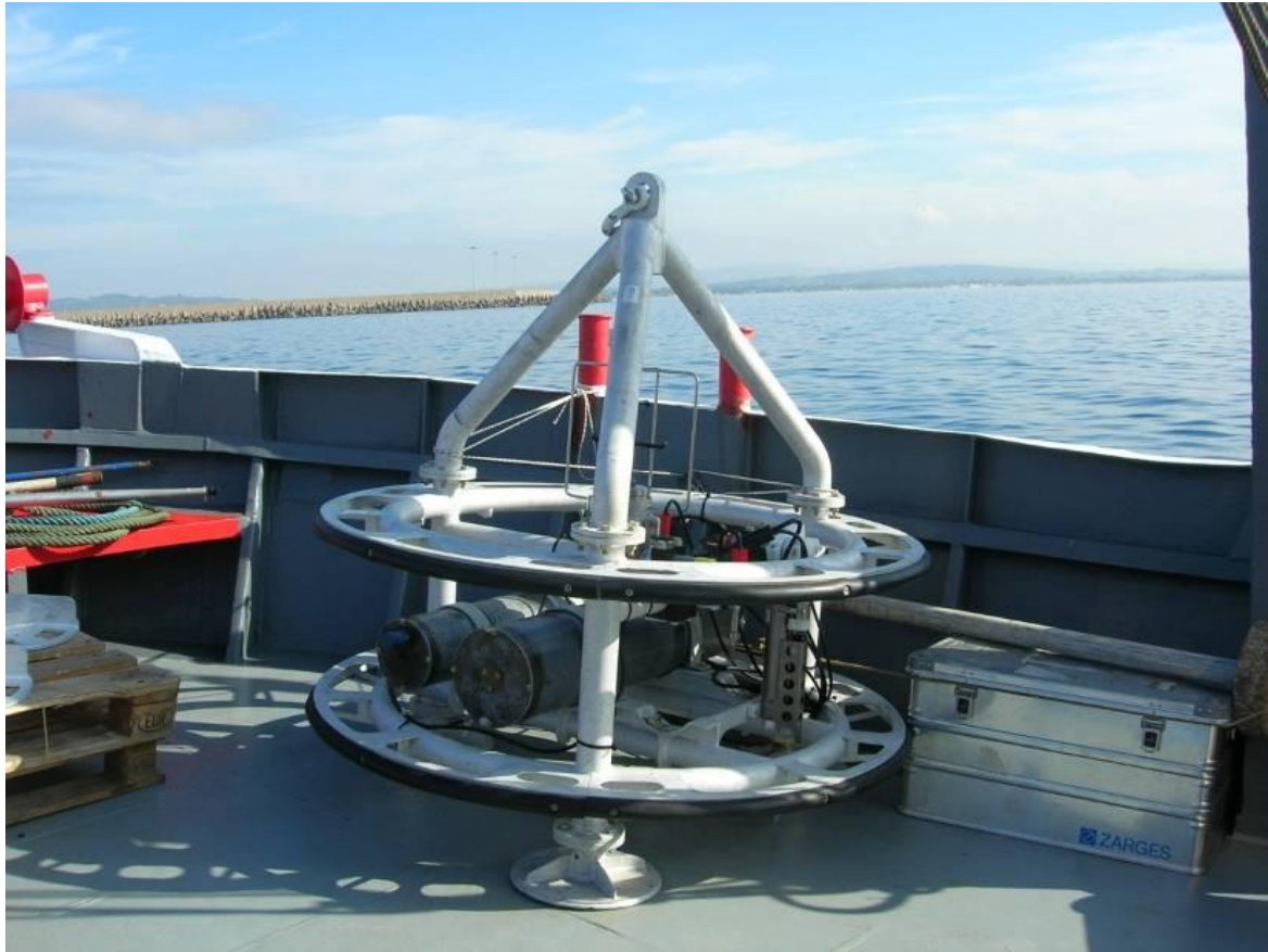
Fig. 2: The GMM benthic observatory on board the research vessel (Barbantonis) in Katakolo Bay.
