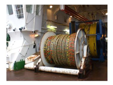
Fig. 8.3: The 600 m long analogue streamer (Type PRAKLA)
