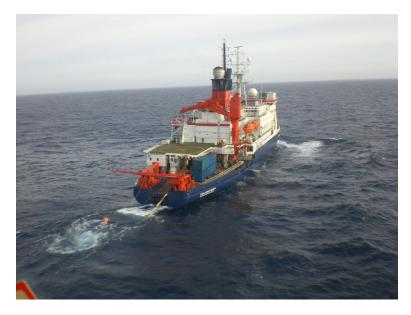
Fig. 8.4: Polarstern with the towed airgun cluster and 600 m streamer taken during a helicopter control flight to check the correct depth position of the streamer.
