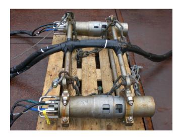
Fig. 8.2: High-frequency 2 GI-Airgun cluster used for the seismic surveys
