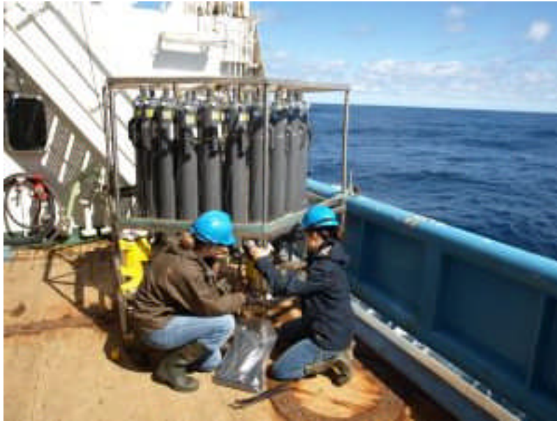
Inge and Lucy busy with attaching the dataloggers to the CTD.
