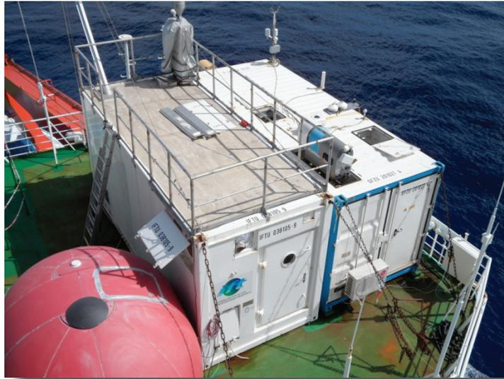
Fig. 3.1.1: Aerosol-Container (left) and OCEANET-Container (right) on the observations deck of *Polarstern* during ANT-XXVII/4
