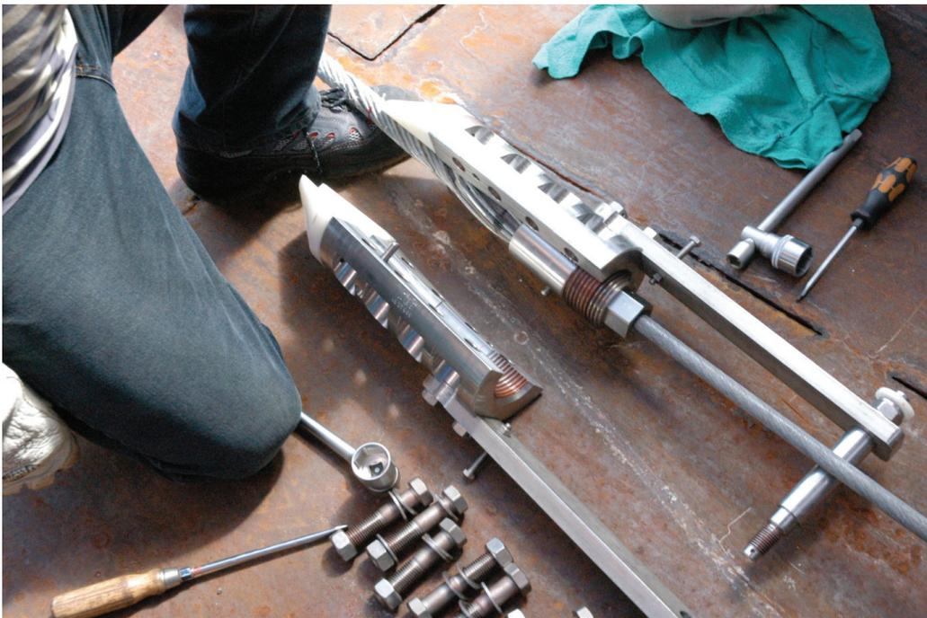
*Fig. 3.9.2: The disassembled “AWI-GRIP®” termination*
