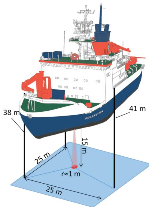
Fig. 3.8.1: Location of deployment of the three underwater winches or 'plumblines' (black vertical lines), respectively, and plain of calibration (blue area). Blue thin lines represent the lines connected to small calibration sphere. The red circle marks the sound beam area (radius ca. 1 m) in 15 m depth underneath the ship.
