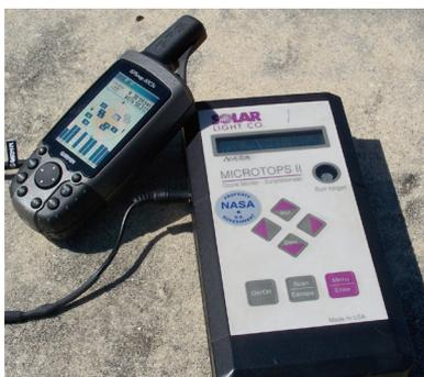
Fig. 3.3.2: Picture of instrument: left GPS, right MICROTOPS
