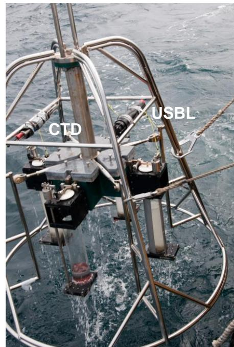
**Figure 6:** MUC retrieval with indication of position USBL transponder and CTD.
