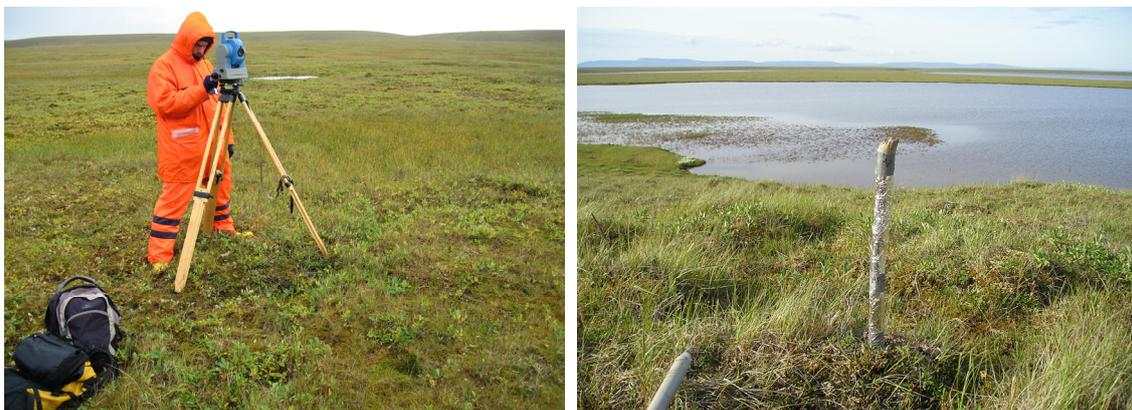
**Figure 9-3:** left) performing stationing, right) marked backside point.
