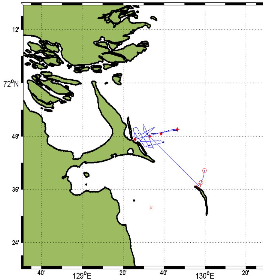
**Figure 11-5:** A map of the region around Tiksi, Yakutia shows the southeastern discharge of the Lena river (top left), the Bykovsky Peninsula and Muostakh Island. Blue lines indicate seismic profiles, red marks indicate datalogger (CT or TD) positions.
