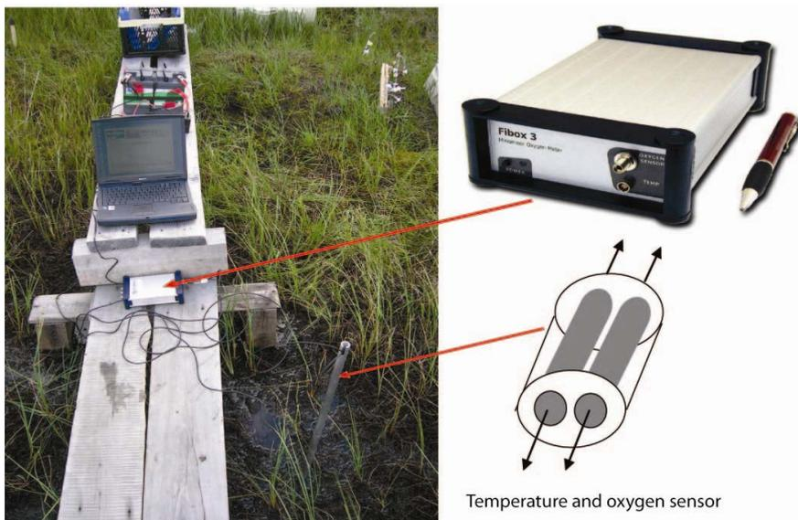
**Figure 3-4:** Setup of optode oxygen sensor in the field.
