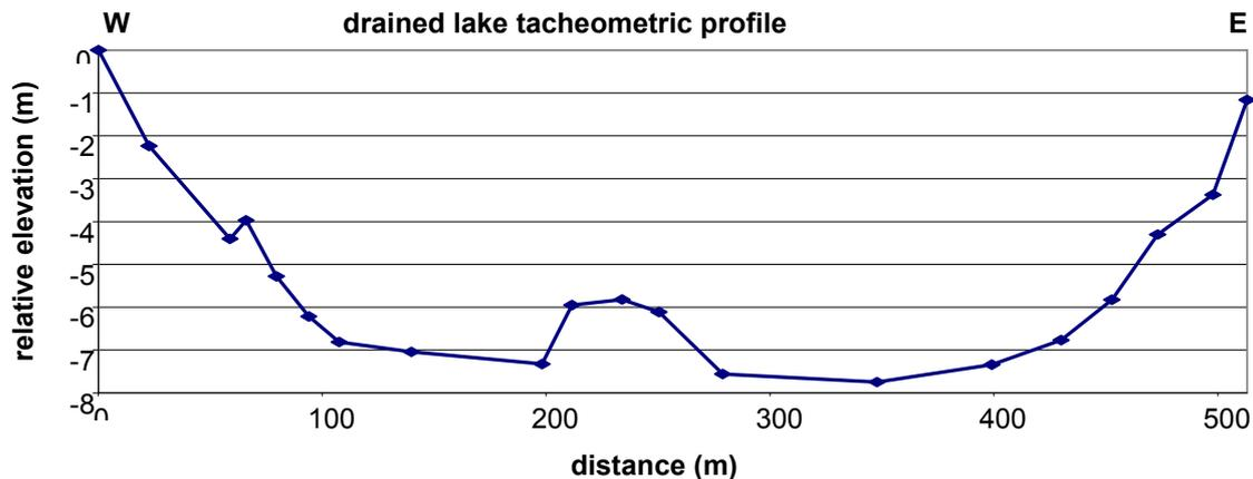
**Figure 9-4:** Tacheometric profile through drained lake basin.
