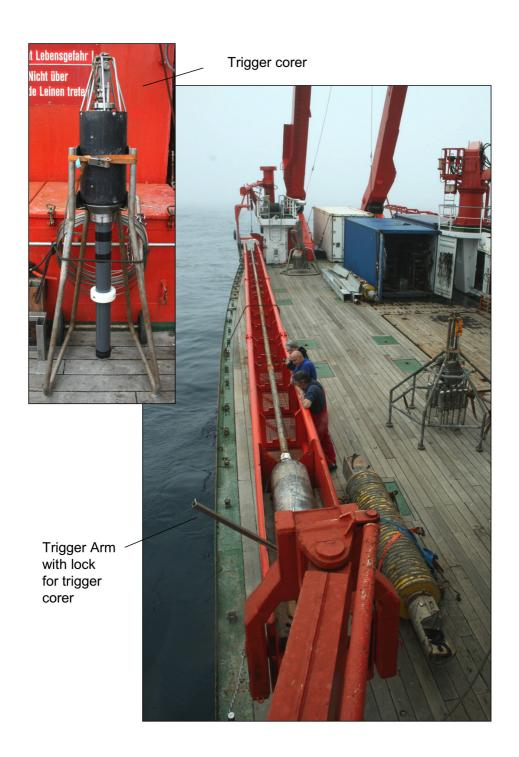
Fig. 3.4-1. The 25 m long piston corer on the R/V Sonne working deck.
