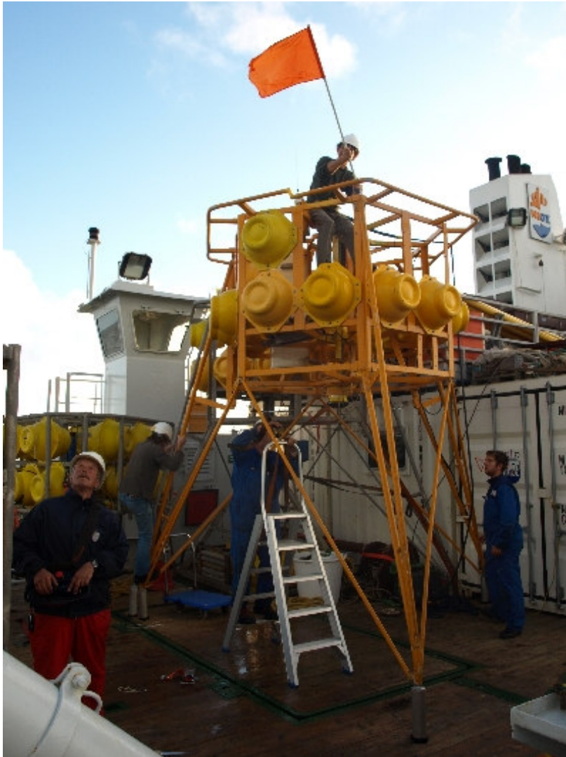
Fig. 8. BOBO lander after being deployed for 7 days in the Belgica Mound area.
