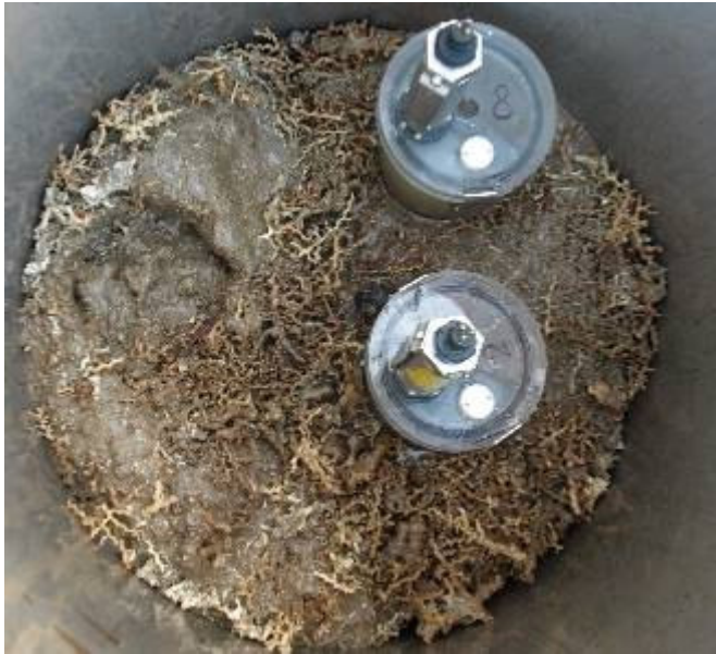
Fig. 4: Boxcore sample with inserted incubation cores.
