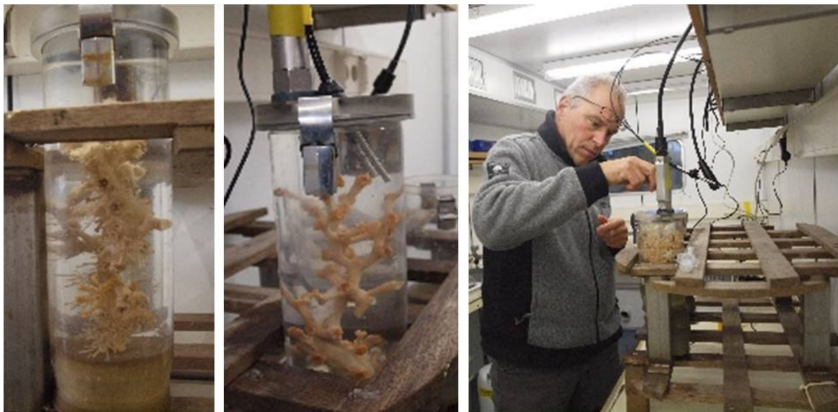
Fig. 5. Incubation cores with animals. Left: white softcoral. Middle: Lophelia . Right: Gerard Duineveld incubating Madrepora . Core with Presence optode, temperature sensor and stirring motor in core holder visible. All measurements done at bottom temperature.
