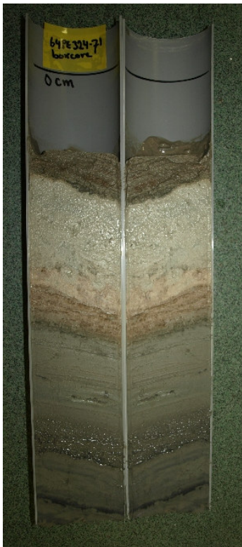
A core from a boxcore sample sliced vertically to show the complicated nature of the layering. Right: the storage container almost half full.
