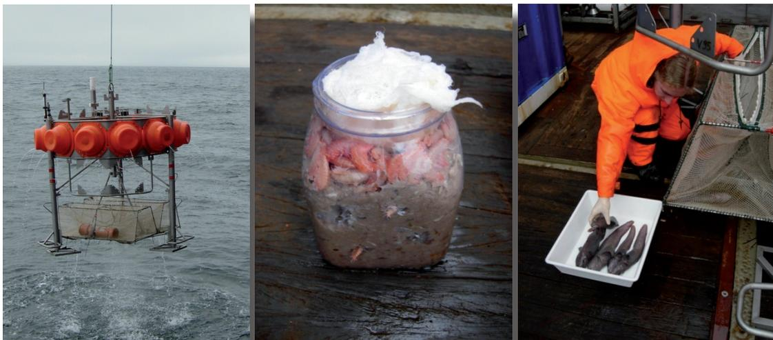
*Fig. 7.4: Recovery of the trap-lander deployed to catch benthic scavengers and demersal fish*
