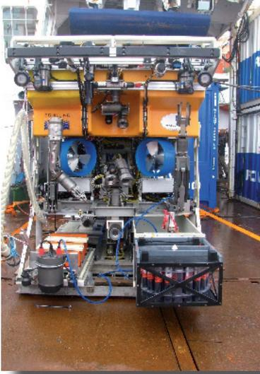
*Fig. 3.1: ROV KIEL 6000 with marker dropper and vertical megacam installed on the toolskid drawers just before station 164ROV04*
