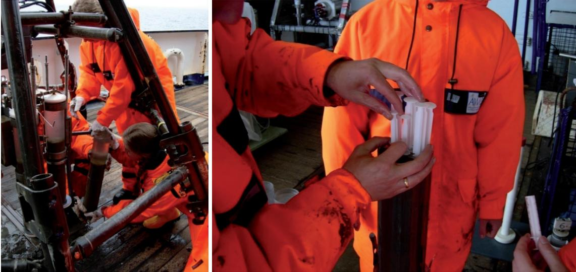
Fig. 7.2: Sampling of undisturbed surface sediments using the multiple corer (MUC)
