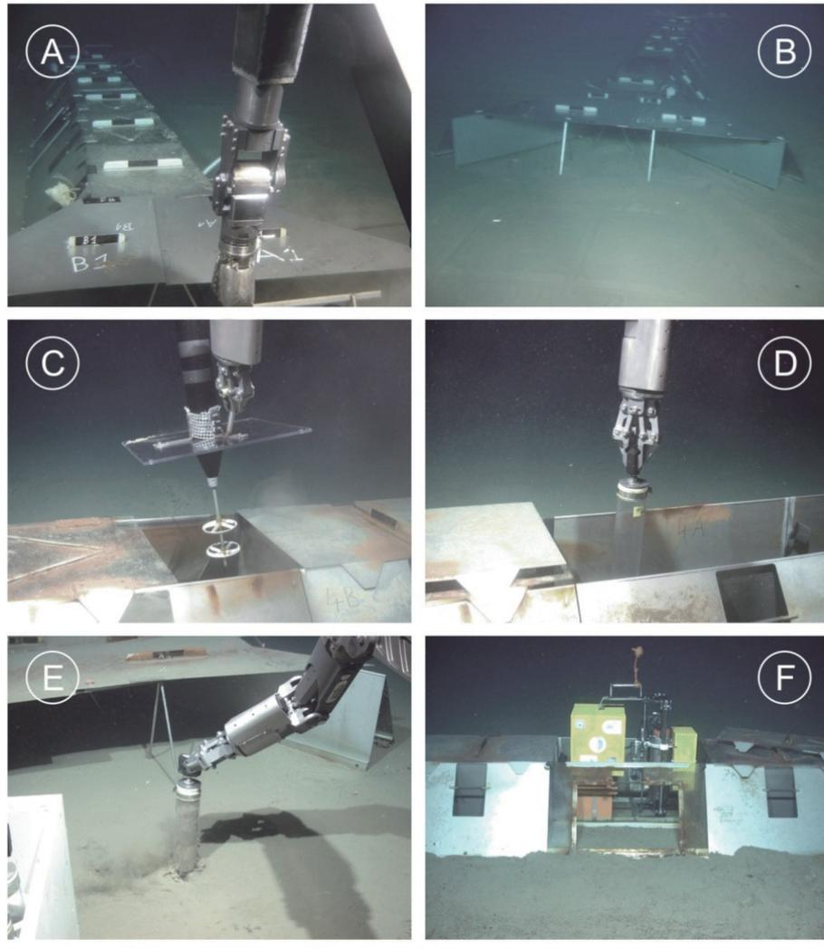
*Fig. 7.8: Experimental flume at the deep seafloor: (A) Installation with the French ROV VICTOR 6000" in 2003; (B) v-shaped inlet to accelerate bottom currents; (C) current measurements using a MAVS-3 acoustical current meter; (D) sediment sampling inside the flume; (E) push-coring of sediments close to the outlet; (F) ROV-handled microprofiler unit inserted into the flume to take oxygen profiles in the uppermost sediment layers*
