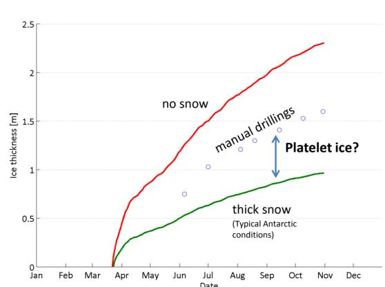
A simple Freezing-Degree-Day model was applied to compare sea-ice thickness as it would result from pure thermodynamic growth with thickness measured in the field (including platelet ice contribution)
