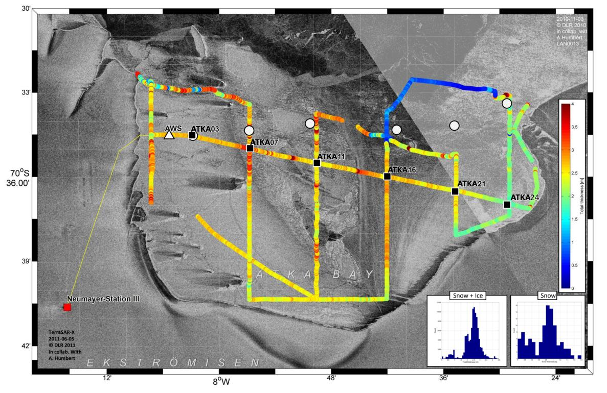
Top: TerraSAR-X image of Atka Bay with stations in 2010 (white) and 2011 (black), where regular manual thickness measurements took place. Station names (e.g. ATKA03) refer to the distance to the western ice-shelf edge. The profile was relocated in 2011 in order to reduce the likeliness of an early ice break-up at ATKA07 as in 2010.
