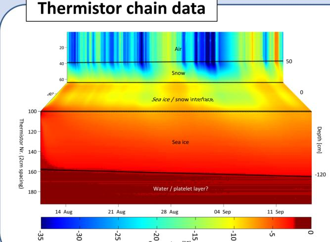
Temperatures measured by a thermistor chain deployed between ATKA03 and the iceshelf edge. Due to technical problems, data is only available for 3 weeks in 2011. Air/snow, snow/sea-ice and sea-ice/water interfaces are visible around 50 cm, 0 cm and -120 cm. Below the solid sea ice, a layer of ice platelets might be recognizable.
