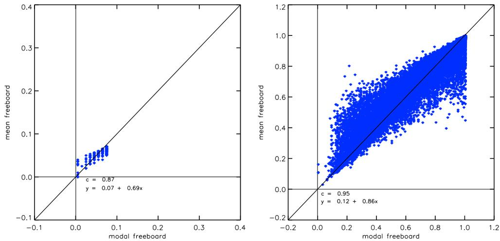
**Fig. D.5:** Comparison between mean and modal sea ice freeboard from laser measurements performed in the western Weddell Sea in February 2010. Left: Freeboards limited to 0.08 m, right: Freeboards limited to 1 m. The black line indicates a slope of 1.
