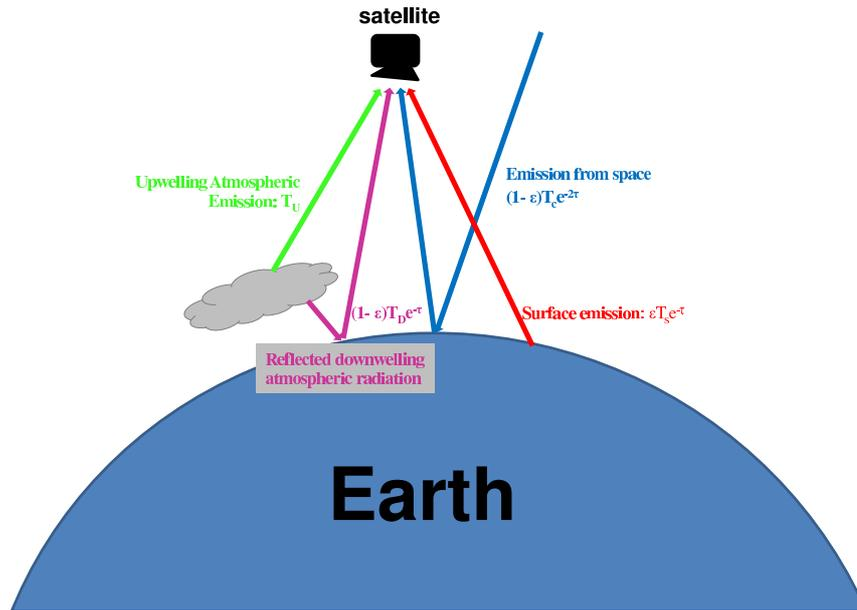
**Fig. A.1:** Scheme of radiative transfer that influences measured brightness temperatures from microwave radiometer data. Redraw based on Swift & Cavalieri (1985).
