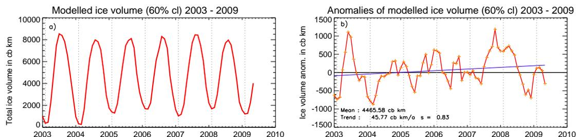
**Fig. 4.20:** Monthly mean simulated sea ice volume and its anomalies in  $\text{km}^3$  for the period from January 2003 till May 2009, corresponding to the ICESat period.
