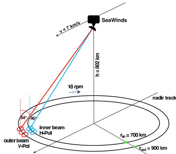
**Fig. 4.1:** Measurement principle of the SeaWinds instrument on-board QuikSCAT (after Spencer et al. (2000) and Ezraty & Piollé (2001)).
