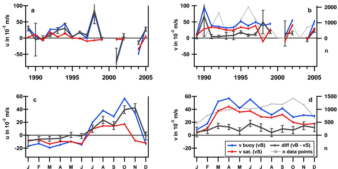
**Fig. 5.7:** Comparison of mean values for zonal (left) and meridional (right) drift velocities derived from buoys (blue) and satellites (red), the average difference between both data sets (gray) with attached 95% confidence interval. The number of corresponding sea ice drift vector pairs ( $n$ ) is shown in light gray (only in Fig. b and d). Upper figures display yearly and lower figures monthly distribution. Figures after Schwegmann *et al.* (2011).
