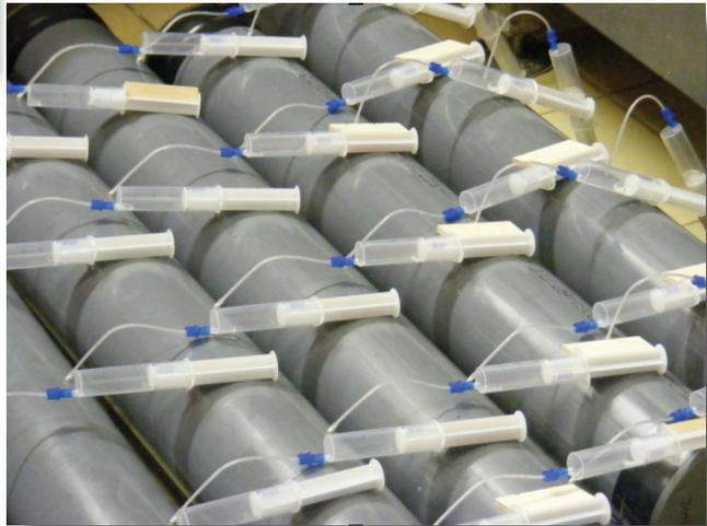
Fig. 8.8: Pore water sampling of GC segments
