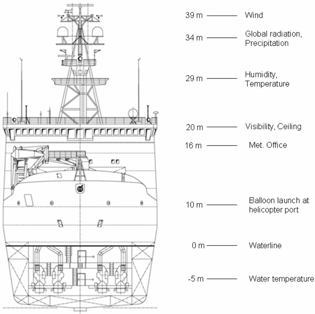
Fig. 1: Heights of the meteorological sensors with respect to the waterline
