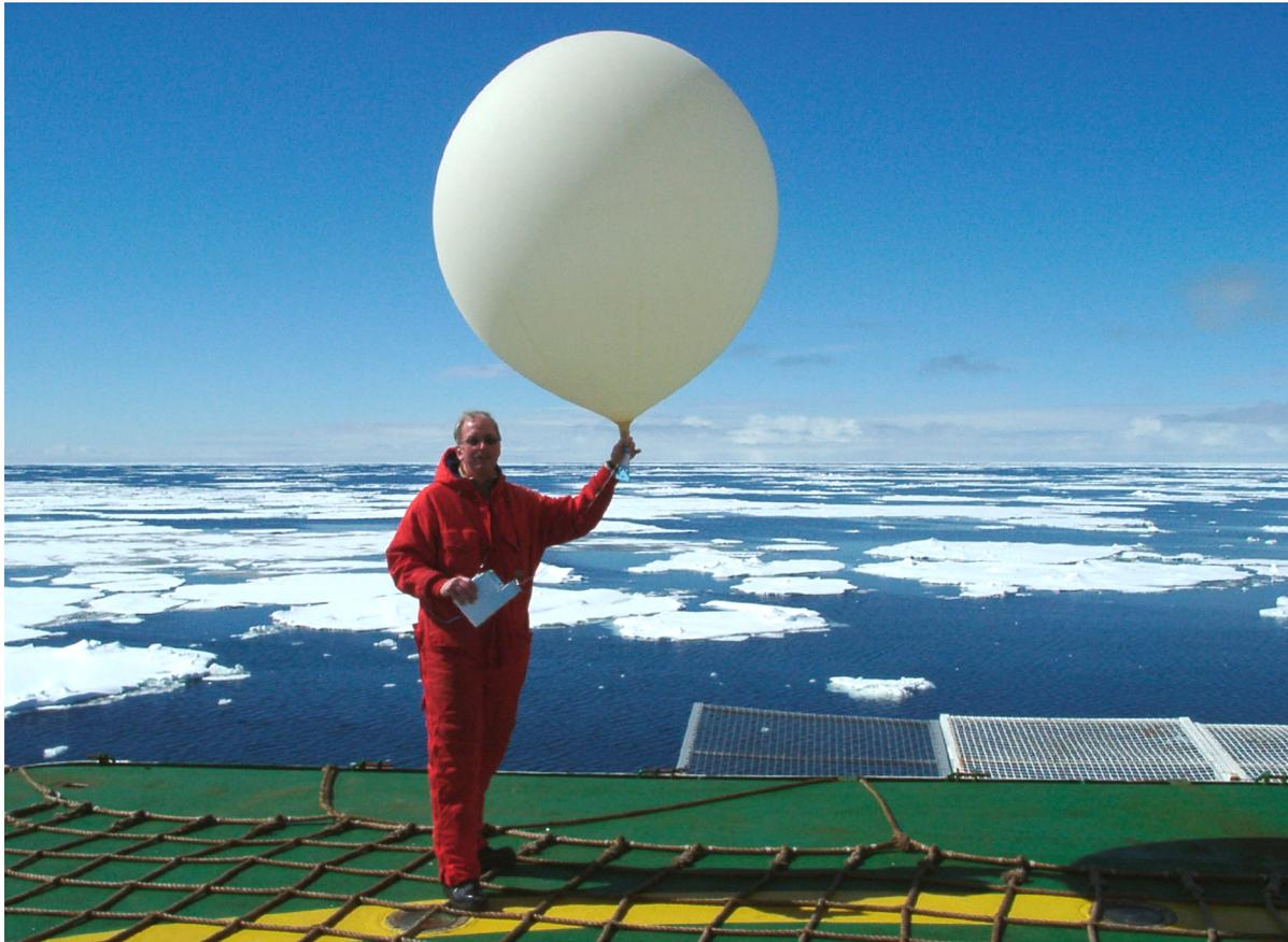
Fig. 2: Balloon launch from the helicopter port of Polarstern
